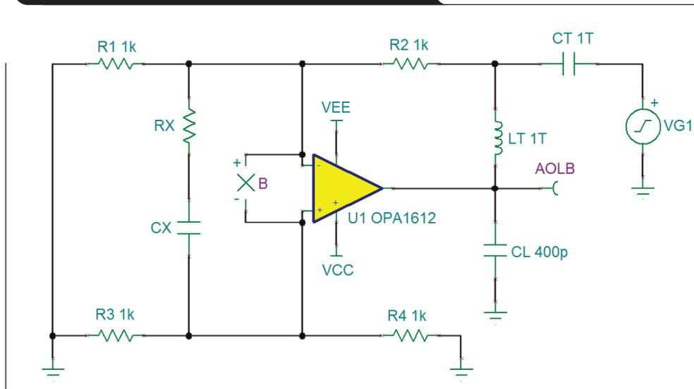
A value of 1.2 nF is very close to the calculated value for  $C_X$ . The resulting zero frequency is:
