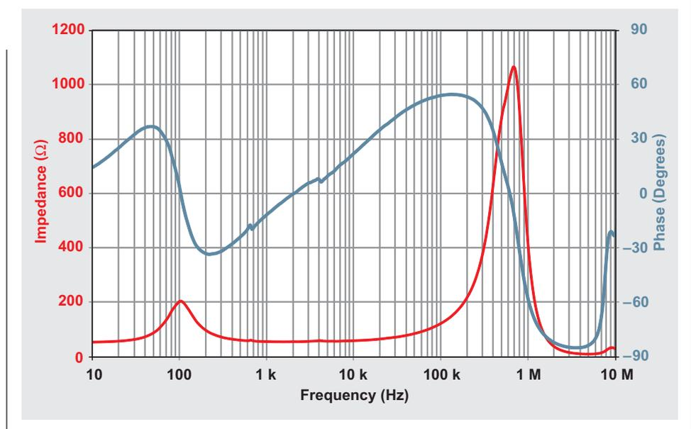
Two resonant peaks are clearly evident in the impedance plot. The low-frequency resonance at 100 Hz is produced by the mechanical and electrical properties of the drivers in the headphones. The high-frequency resonance is created from the interaction of the cable
