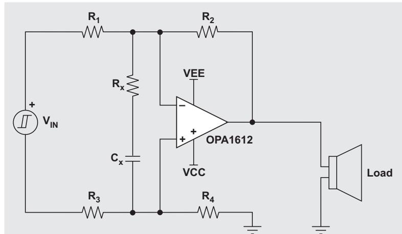
(a) Amplifier circuit with  $R_X/C_X$  network
