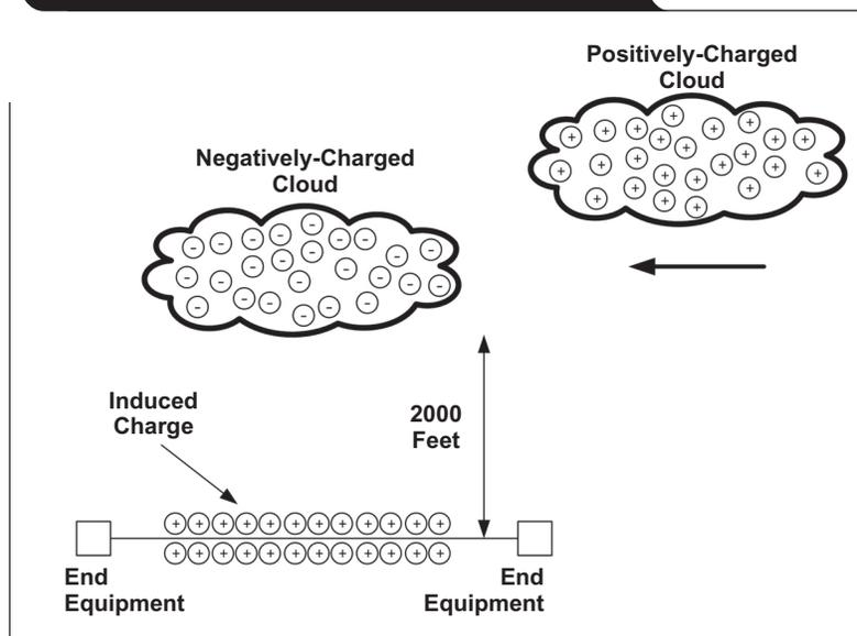
**Figure 2. A cross-strike event may result in damage to end equipment**
