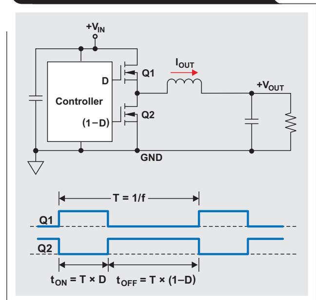
**Figure 2. Simplified negative synchronous boost regulator**
