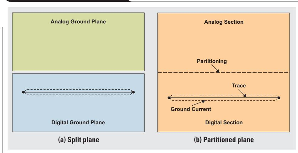
into analog and digital sections (see Figure 4b). Analog signals must be routed only in the board's analog section, and digital signals must be routed only in the board's digital section, with both on all layers. Under these conditions, the digital return currents do not flow in the analog section of the ground plane and remain under the digital signal trace. Figure 4 compares a split plane and a partitioned plane.
