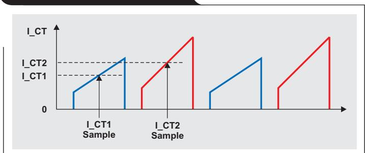
With proper sampling of the CT currents, the cycle-by-cycle approach gives good current balancing. Figure 4 shows test results from a 360-W, digitally controlled interleaved PFC. As can be seen, there is a big difference between the inductor currents, but they almost overlap after being balanced.
