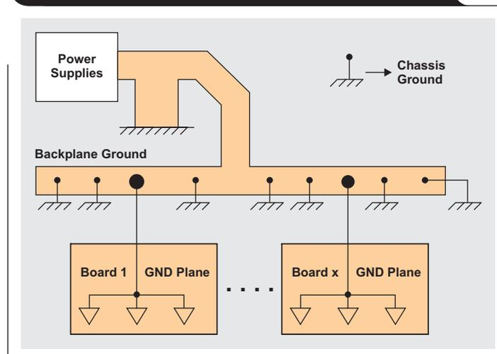
ground impedance is maintained all the way through the PCBs, the backplane, and ultimately the chassis. However, it is critical that good electrical contacts be made where the grounds are connected to the sheet-metal chassis. This requires self-tapping sheet-metal screws or biting washers. Special care must be taken where anodized aluminum is used for the chassis material, since its surface acts as an insulator.
