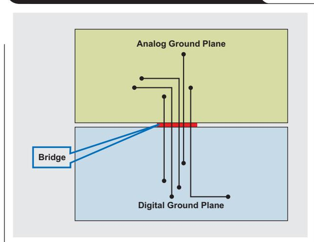
**Figure 4. Ground-plane layouts**
