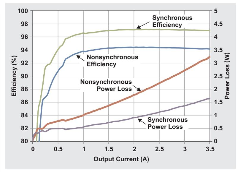
**Figure 4. Measured efficiency and power loss in a high-duty-cycle application**
