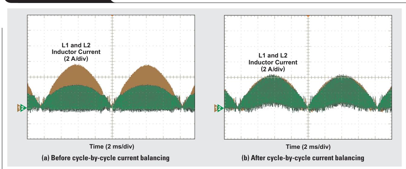
**Figure 5. AC input current**
