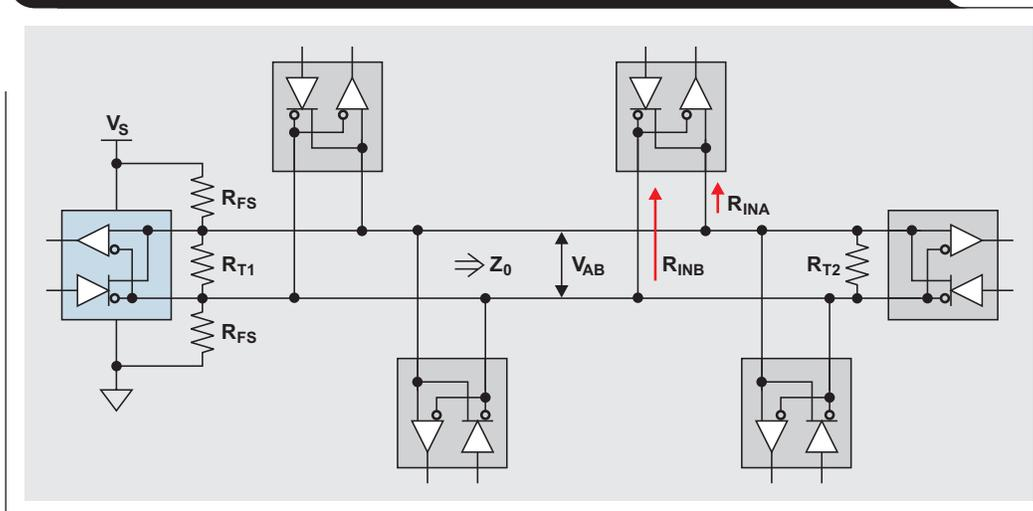
commonly installed at the master end of the bus, while the other cable end receives a termination resistor ( $R_{T2}$ ) matching the characteristic line impedance ( $Z_0$ ).
