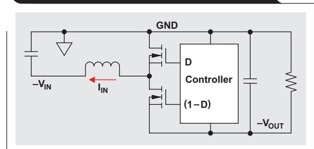
Figure 3. Complete schematic of the example negative boost regulator
