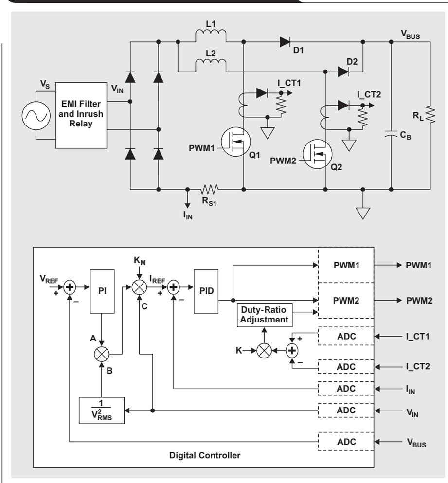
output, which is also positive, increases the duty ratio of phase 2 and thus its current. This configuration is shown in Figure 2.
