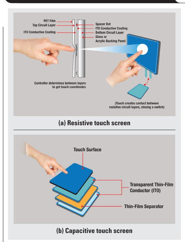
Figure 2. ITO rows and columns are overlaid to make one full sensor sheet
