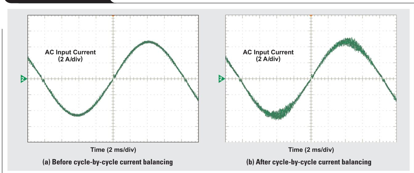
the same duty-ratio adjustment is applied to the next half AC cycle. This essentially solves the issue of high-frequency noise. Test results showed that the AC current's waveform was almost the same as before current balancing was enabled; the high-frequency noise went away.
