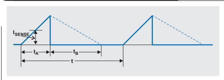
For a boost-type converter in steady-state operation, the volt-second of the boost inductor maintains balance in each switching period:
