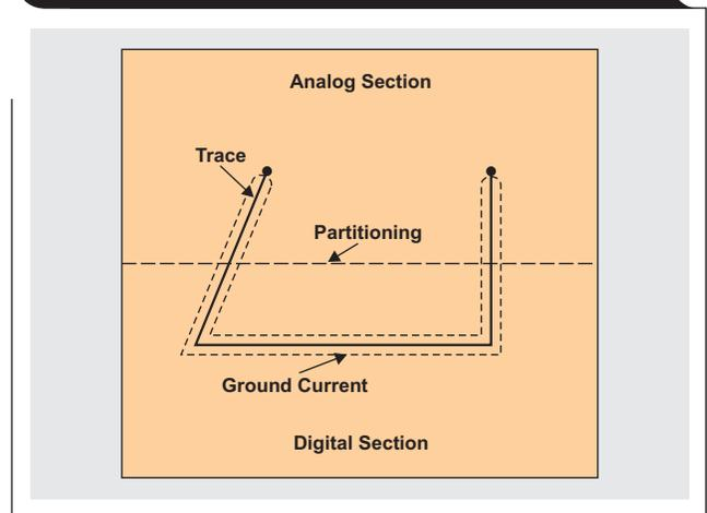
**Figure 6. Grounding mixed-signal devices on a single PCB**
