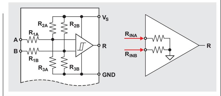
Because  $R_{FS}$  in combination with  $R_{INEQ}$  makes up the total common-mode load for a signal line, the parallel value of the two must not exceed the specified maximum of  $375\ \Omega$ , which is expressed through
