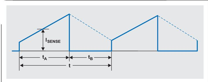
**Figure 9. Sensed current waveform at DCM**
