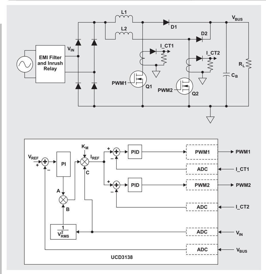
higher-speed CPU. Figure 7 shows the configuration of these dual control loops implemented with the UCD3138. The current-feedback signal from each phase needs to be measured. Normally, a CT placed above the MOSFET can be used. Since no current shunt is needed, this configuration also can improve efficiency.
