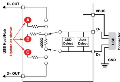
Figure 3. USB charging Controller Handshake Interface
