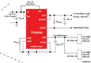
Figure 1. TPS2500 Application Diagram
