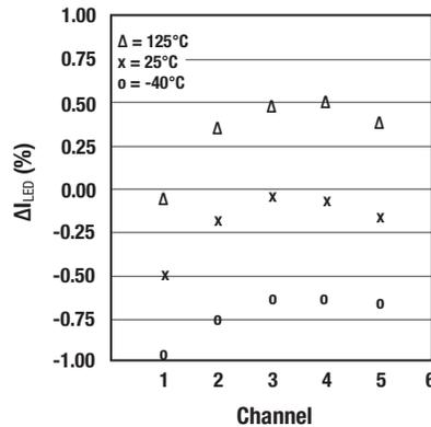
Current regulation (channel-to-channel) vs temperature.
