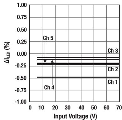
Current regulation (channel-to-channel) vs  $V_{IN}$ .
