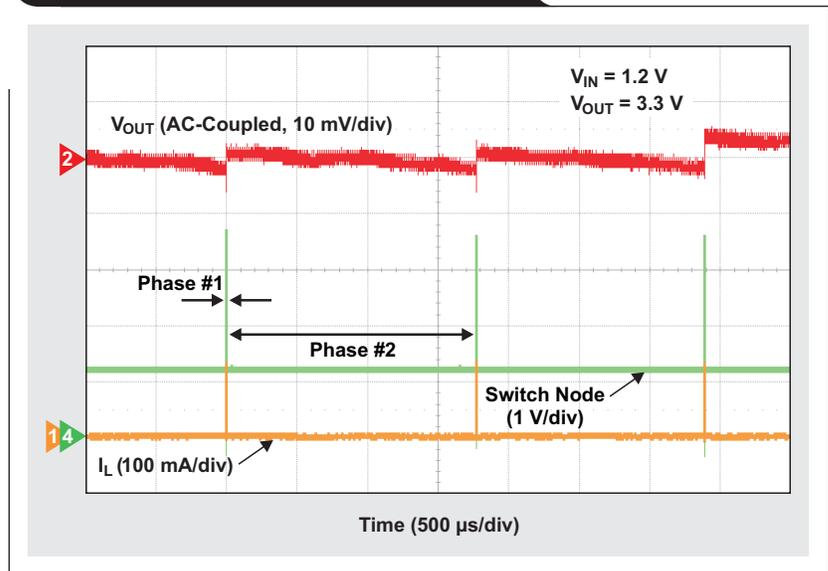
**Figure 3. Switching pulse of TPS61220 during no-load operation**
