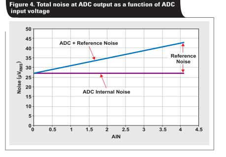
to measure the noise close to both the negative full scale and the positive full scale. Figure 4 shows the results of measuring the reference noise and the ADC noise in a system. These results show that the overall noise is not constant but linearly dependent on the ADC's analog input voltage. When this type of system is designed, it is important to keep the reference noise lower than the ADC's internal noise.
