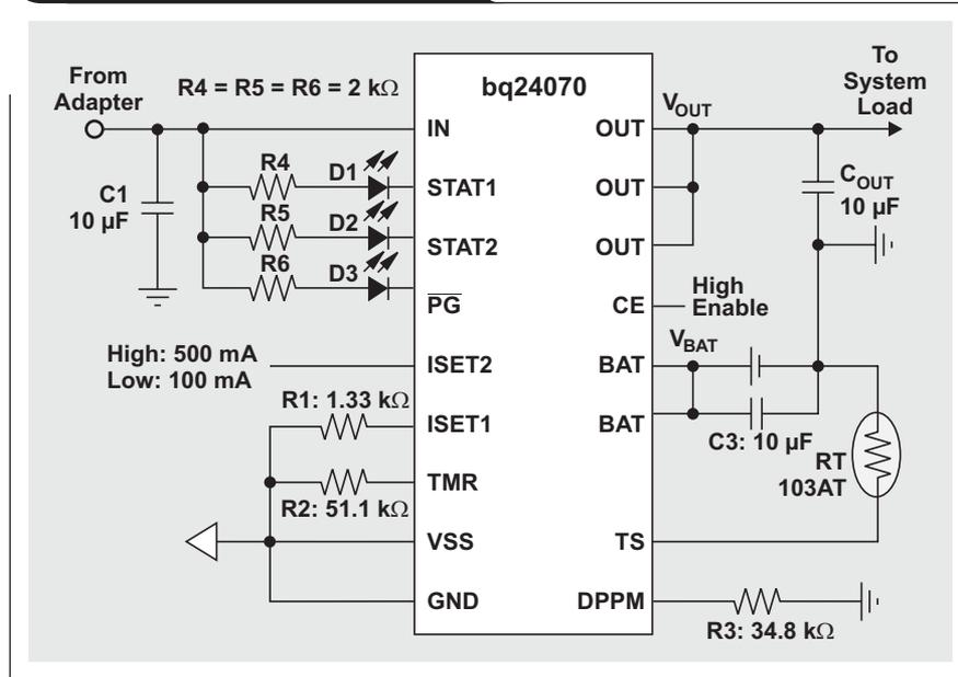
Figure 3 shows an example DPPM Li-Ion battery charger. A thermal regulation loop reduces the charge current to prevent the silicon temperature from exceeding 125°C. Whenever the charge current is reduced because of active thermal regulation or active DPPM, the safety timer's precharge time is automatically increased to eliminate a false safety-timer expiration.
