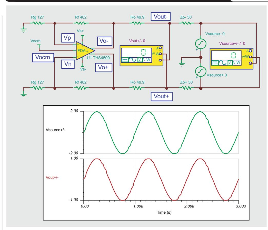
**Figure 7. TINA-TI simulation of FDA output impedance with synthesized impedance-matching resistors**
