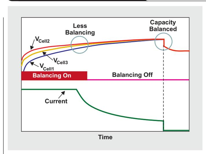
**Figure 7. Principle of external passive cell balancing**
