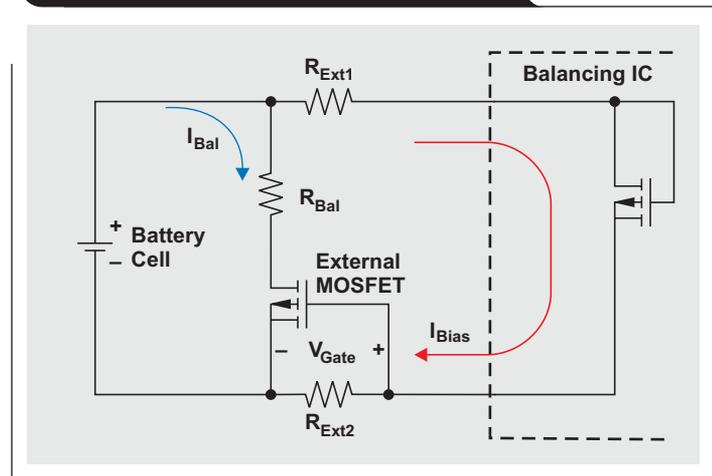
The drawback of this method is that balancing cannot be performed on adjacent cells at the same time (see Figure 8a). This is because, when adjacent internal FETs are turned on, there is no current flowing through  $R_{Ext2}$ , so Q1 remains off even when the internal switch is enabled. In practice, this is not an issue because the fast external cell balancing can quickly balance the cell associated with Q2, and then the cell associated with Q1 will be balanced.
