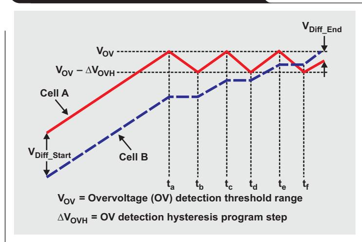
**Figure 3. Simple voltage-based cell balancing may not effectively balance capacity**
