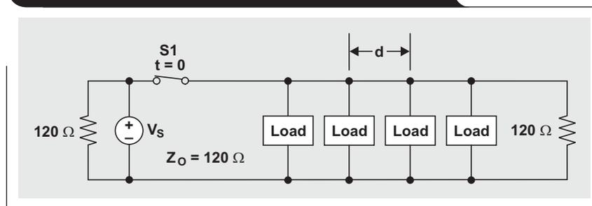
**Figure 2. Minimum distance required between CAN nodes**
