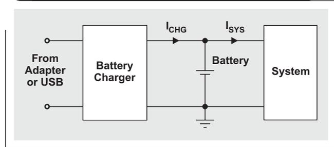
**Figure 2. Simplified block diagram of PPM battery charger**
