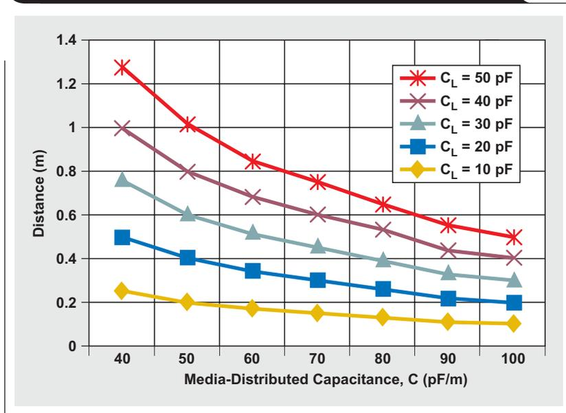
The minimum safe distance between nodes,  $d$ , is a function of the device lumped-load capacitance,  $C_L$ , and the cable's distributed capacitance per unit length,  $C$ , where  $d > C_L/0.98 C$  meters (if  $C$  is in pF/m) or feet (if  $C$  is in pF/ft). Figure 2 displays this relationship graphically. For a complete development of this equation, please see Reference 1.
