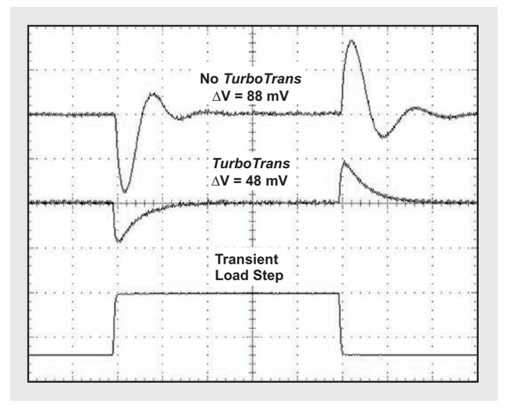
response to a load step is shown with and without the *TurboTrans* feature.
