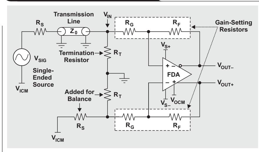
**Figure 5. FDA with AC-coupled RF/IF/CATV amplifier input**
