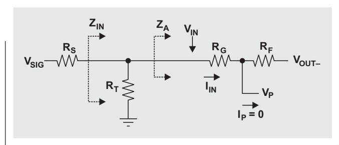
**Figure 8. Thevenin equivalent of positive side**
