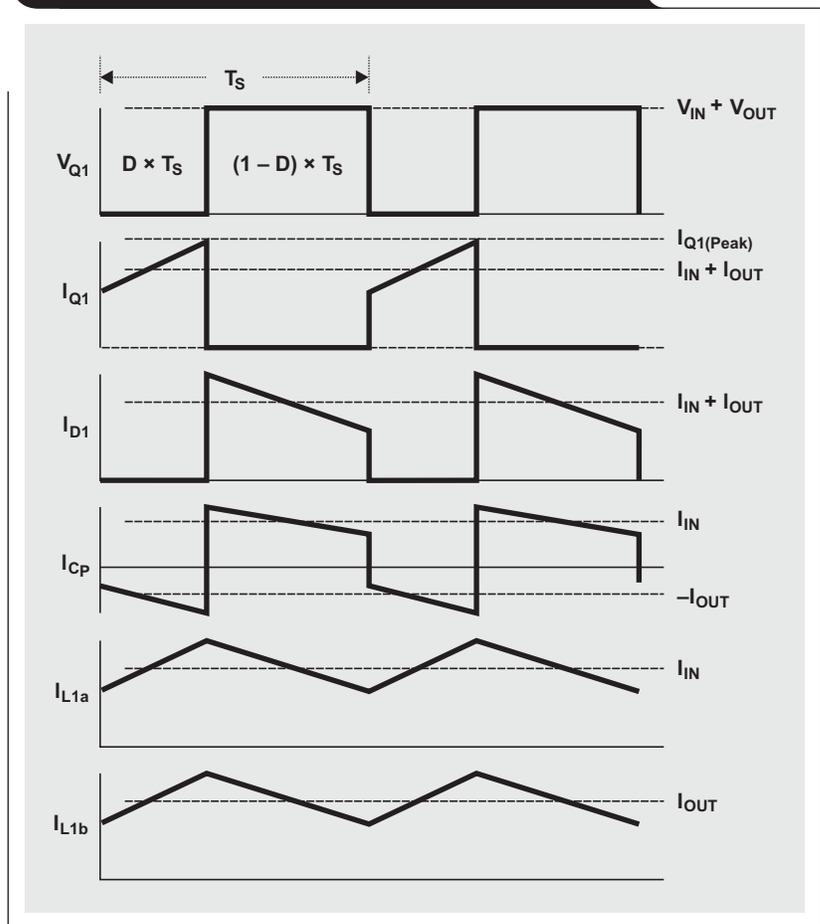
not have equal inductance and the ripple currents will not be exactly equal. Regardless, for a desired ripple-current value, the inductance required in a coupled inductor is estimated to be half of what would be needed if there were two separate inductors, as shown in Equation 4:
