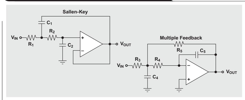
The filter-response DC gain in Figure 2 is equal to 0 dB. The corner frequency of this low-pass filter occurs at 1 kHz, and the gain magnitude at 1 kHz is equal to -3 dB. Following this corner frequency, the filter response falls off at a rate of -40 dB/decade. Theoretically, the attenuation continues to occur as the frequency increases.
