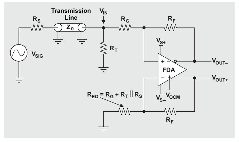
**Figure 7. Positive side of FDA circuit**
