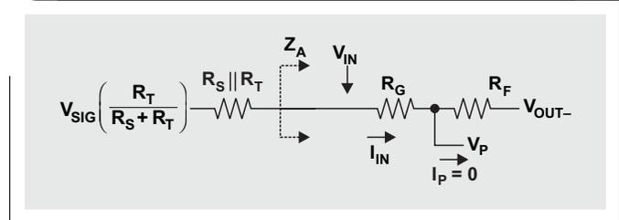
equation for only the amplifier's AC or signal response to  $V_{OUT-}$ , which we will call  $V_{OUT- (AC \text{ only})}$ :
