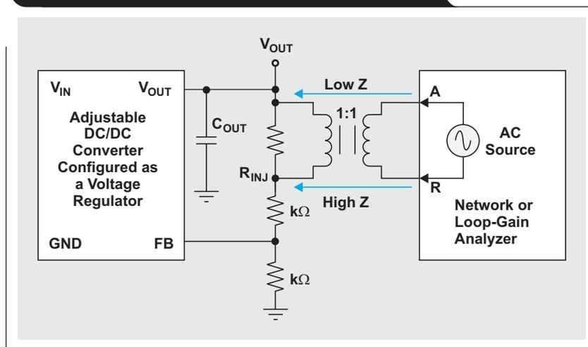
In a current-regulating configuration, with the load itself being the upper FB resistor, the injection resistor cannot be inserted in series with the LEDs. The converter's operating point must first be changed so the resistor can be inserted between the FB pin and the sense resistor as shown in Figure 6. In some cases, a non-inverting, unity-gain buffer amplifier may be necessary to lower the impedance at the injection point and reduce measurement noise.
