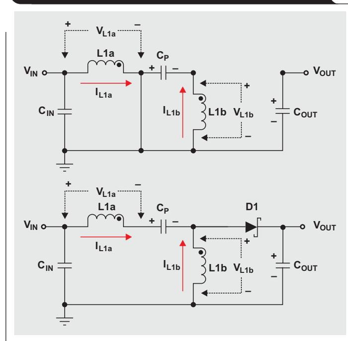
capacitor  $C_P$  is charged to the input voltage,  $V_{IN}$ . Knowing this, we can easily determine the voltages as shown in Figure 3.
