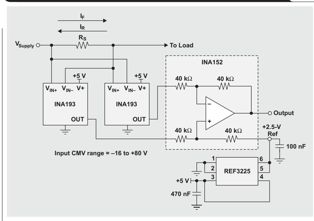
flow in the correct direction. Two of the unidirectional current-shunt-monitor ICs may be interconnected to form a bidirectional current-shunt monitor with a CMV range that extends from -16 to +80 V. The addition of the INA152 instrumentation amplifier and +2.5-V reference completes the circuit. A circuit schematic for the INA193 bidirectional current-shunt monitor is shown in Figure 2.
