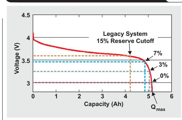
*Track* system, which can provide up to 99% accuracy, we can program the terminate voltage ( $V_{\text{Term}}$ ) at which zero capacity is defined. If we have true 99% accuracy, then the 14% capacity we gain back can be used to significantly increase the run time of the system (see Figure 4).
