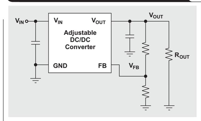
**Figure 2. Adjustable DC/DC converter used to regulate current through LEDs**
