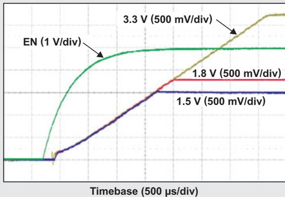
(a) Pseudo power-up sequencing with  $V_{IN}$  connected to 1.8-V output
