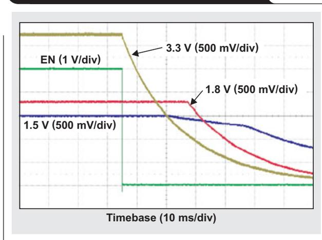
**Figure 4. TPS74301 1.5-V output with power-down sequencing**
