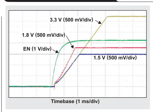
**Figure 3. TPS74301 1.5-V output without power-down sequencing**
