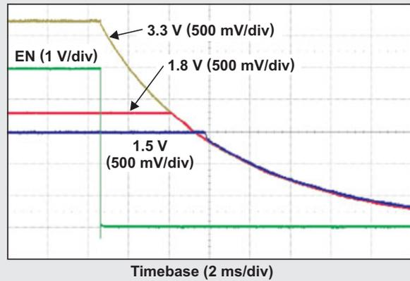
(b) Pseudo power-down sequencing with  $V_{IN}$  connected to 1.8-V output
