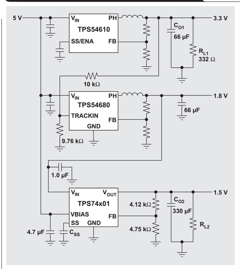
**Figure 6. TPS74801 1.5-V output with  $R_{L2} = 1 \Omega$**
