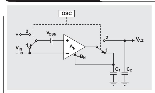
Figure 11. Chopper principle
