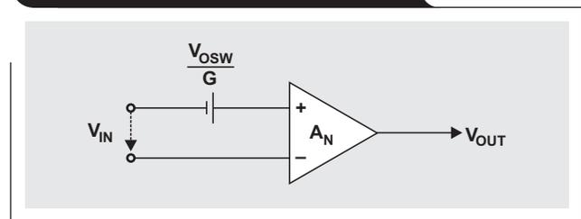
Thus, the DC gain has increased by factor  $G$ , from  $A_W$  to  $A_N$ , while the input offset of the wideband amplifier is reduced by  $G$  (typically 60 dB).
