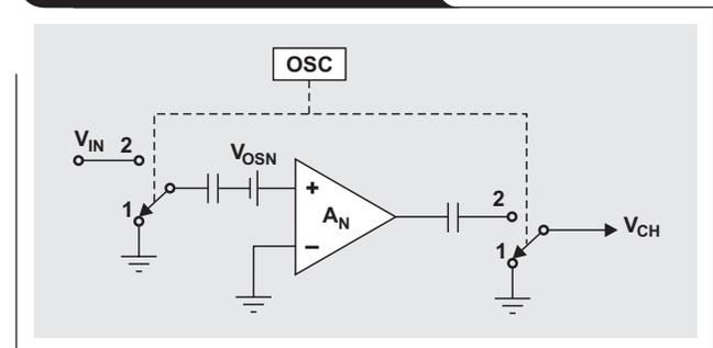
Figure 12. Auto-zeroing and chopping effects on baseband noise
