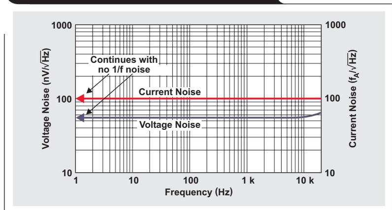
With typical values for offset and drift of  $V_{OS} = 2 \mu\text{V}$  and  $dV_{OS}/dT = 20 \text{ nV}/^\circ\text{C}$ , respectively, the OPA333 also generates only  $1.1 \mu\text{V}_{pp}$  of instantaneous noise in the 0.01- to 10-Hz band. The device offers rail-to-rail input and output and is available in SC70 and SOT23 packaging. Operation is specified from  $-40^\circ\text{C}$  to  $125^\circ\text{C}$ .
