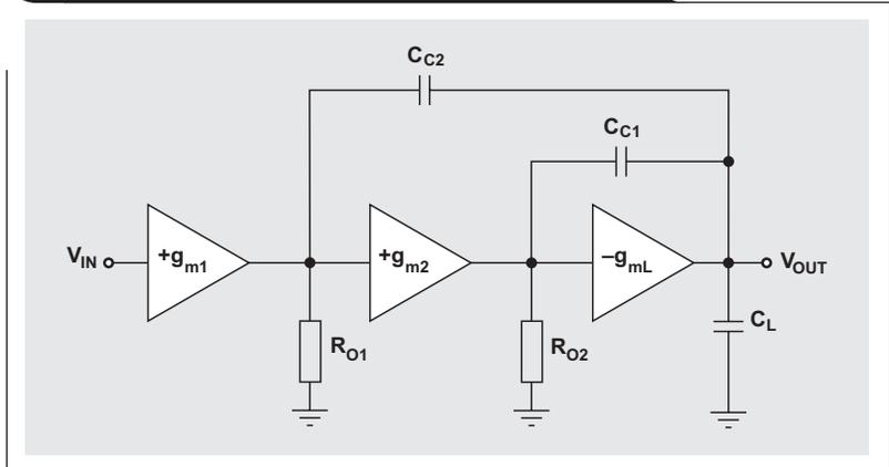
**Figure 8. Pole splitting of the three-stage NMC amplifier**
