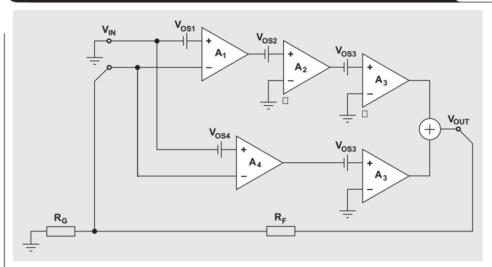
Providing each amplifier with its individual input offset voltage and setting  $V_{IN}$  to zero yields an output of
