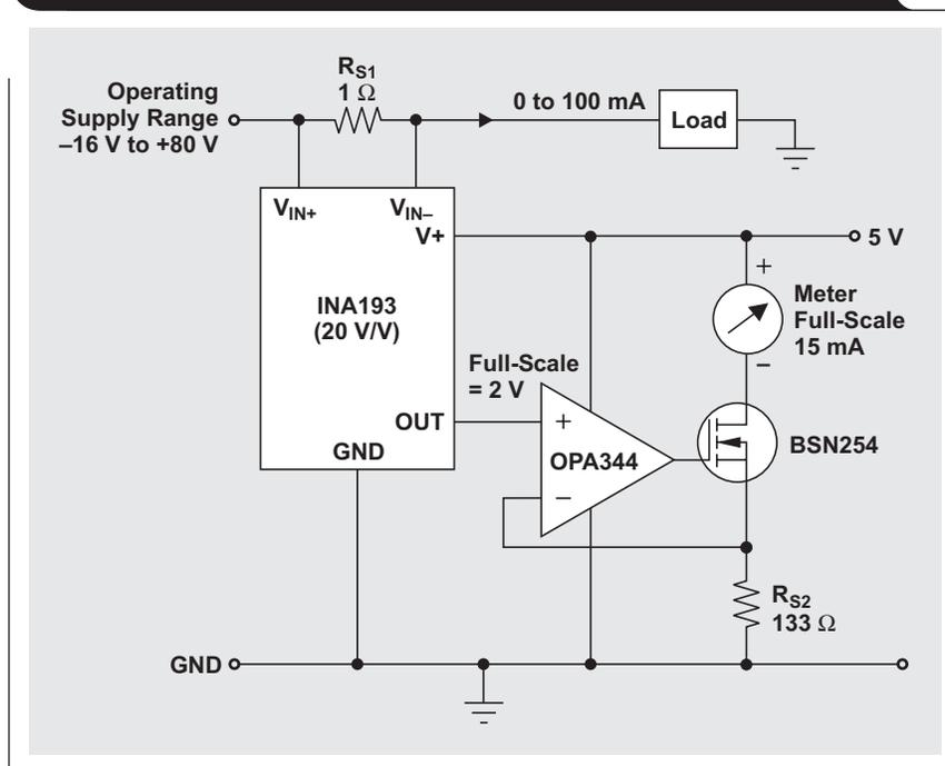
low- $V_{GS}$  requirement. Because the voltage at the non-inverting OPA344 input equals the one at the inverting input, the full-scale output of 2 V lies across  $R_{S2}$ . To allow for the maximum deflection current to flow,  $R_{S2}$  is calculated via
