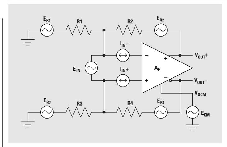
$E_{OD}$  is the differential RMS output noise voltage.  $E_{OD} = A(E_{ID})$ , where  $E_{ID}$  is the input noise source, and A is the gain from the source to the output. Half of  $E_{OD}$  is attributed to the positive output ( $+E_{OD}/2$ ), and half is attributed to the negative output ( $-E_{OD}/2$ ). Therefore,  $(+E_{OD}/2)$  and  $(-E_{OD}/2)$  are correlated to one another and to the input source, and can be directly added together; i.e.,
