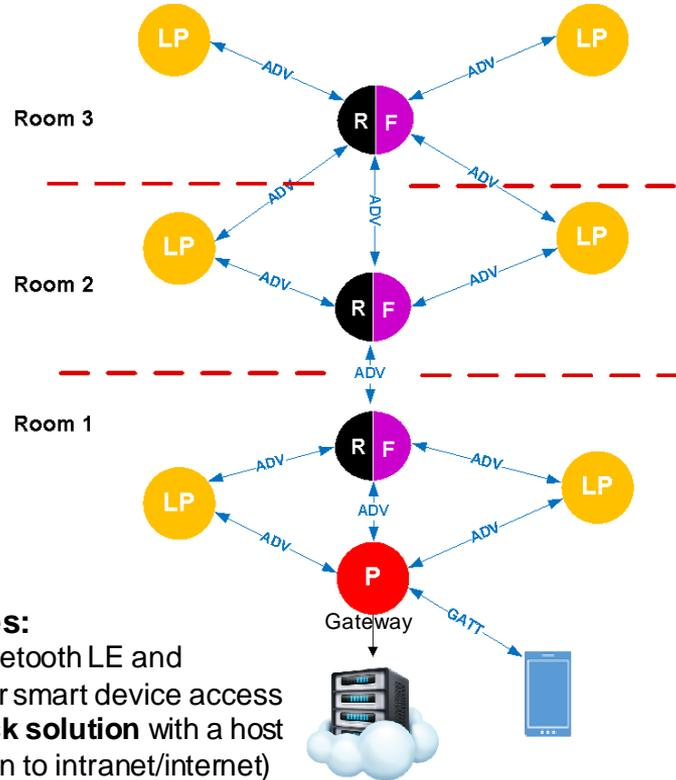
*Wireless sensors operate as low power nodes - transmit sensor data at regular intervals to proxy/gateway or when sensor crosses threshold value.*
