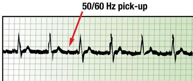
Alternating Current (AC) Interference
