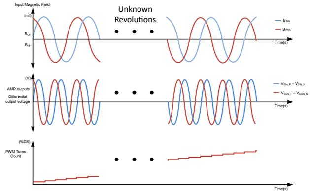
**Figure 4. Turns Counting Through Inactive Sample Period**
