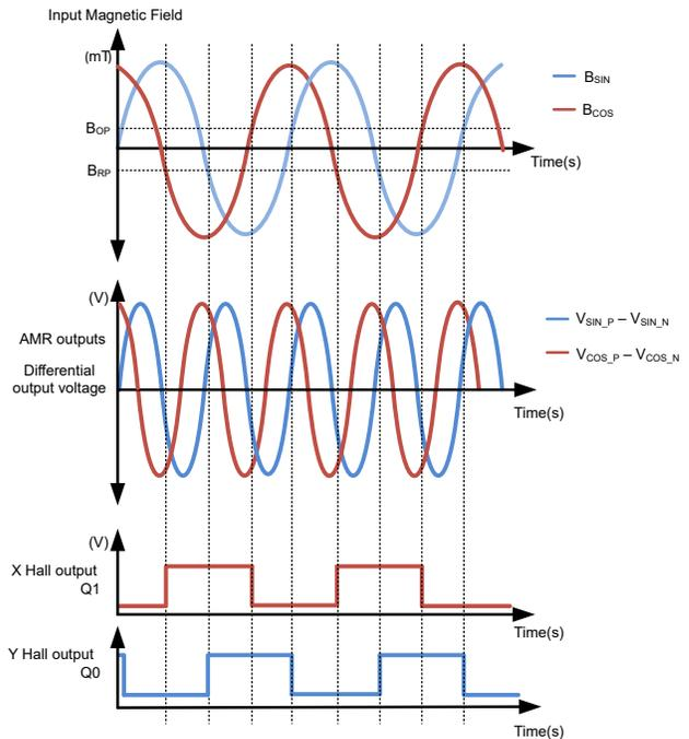
Figure 2. TMAG6180 Sensor Behavior
