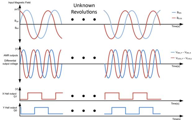
**Figure 3. Unknown Revolutions after Inactive Sample Period**
