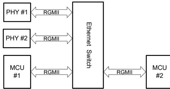
Figure 2. Multicore RGMII Communication
