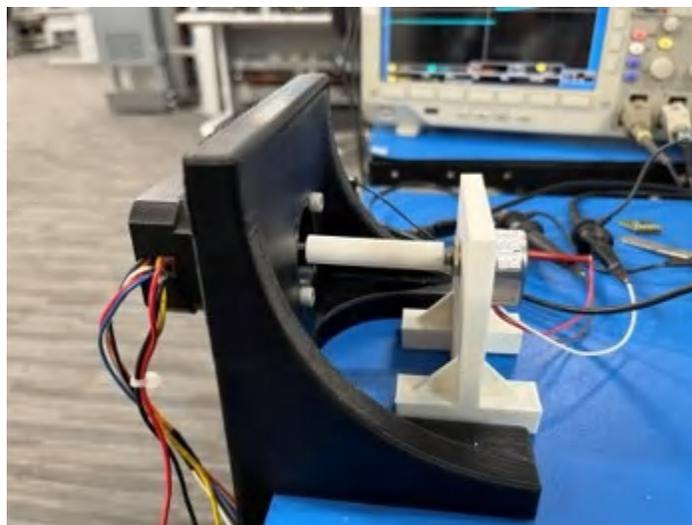
**Figure 4. Motorized Encoder Test Setup**
