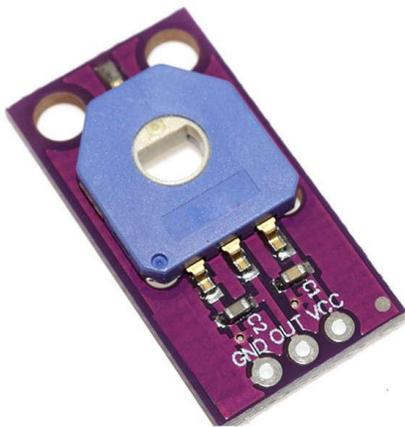
Figure 1. HW-526 Electronic Angle Sensor Module
