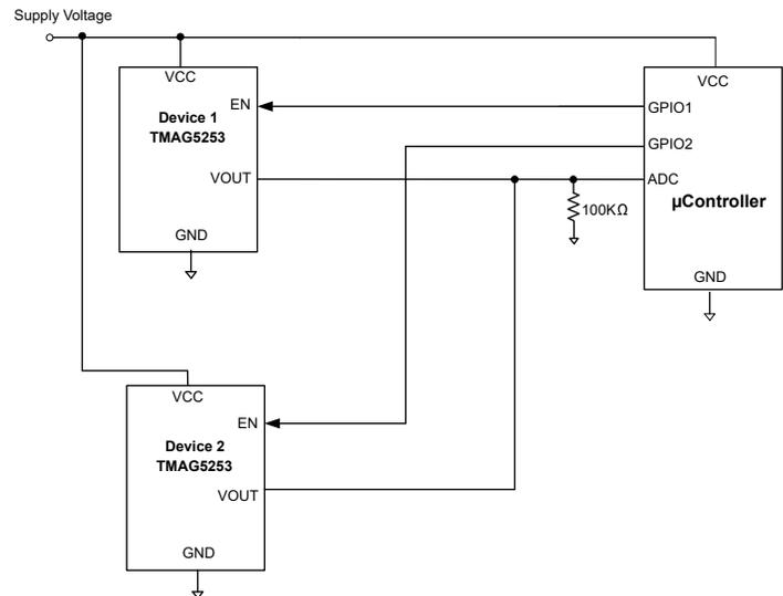
Figure 2. Duty Cycled Sensors
