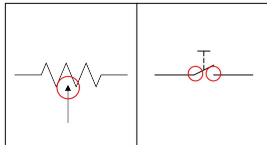
Figure 2. Common Mechanical Failure Points
