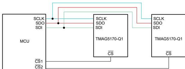
**Figure 6. Simplified Block Diagram**
