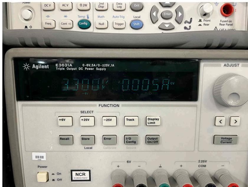
Figure 8-4. TMA5111 Encoder Current Consumption
