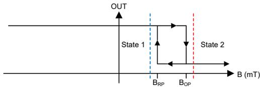
**Figure 3. Unipolar Switch Operation**
