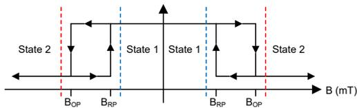
**Figure 2. Omnipolar Switch Operation**
