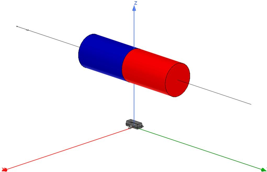
**Figure 2-1. DRV5055 Magnet Orientation for Linear Stroke Detection**
