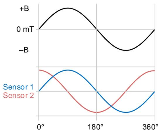
Figure 7. Output from Two Linear Hall Sensors
