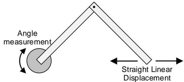
Figure 4. Linear Displacement in a Straight Line
