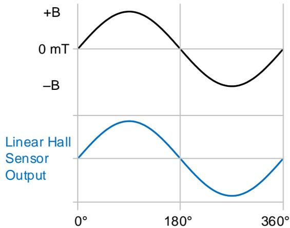
Figure 6. Output from One Linear Hall Sensor
