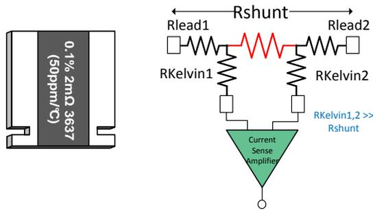
**Figure 2. 4-wire Kelvin Shunt electrical resistance representation**
