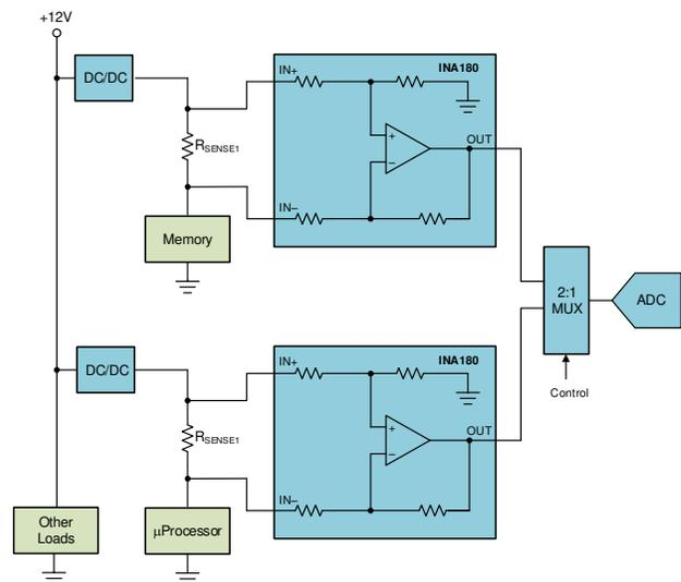
**Figure 2. Monitoring Total Current in Two Supply Rails**
