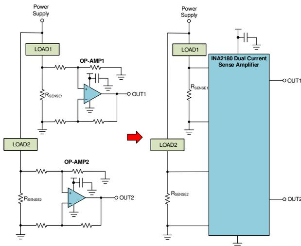
**Figure 1. Discrete vs. Integrated Current Sensing Solutions**
