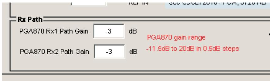
Figure 24. TSW3725 GUI – RX Path Gain
