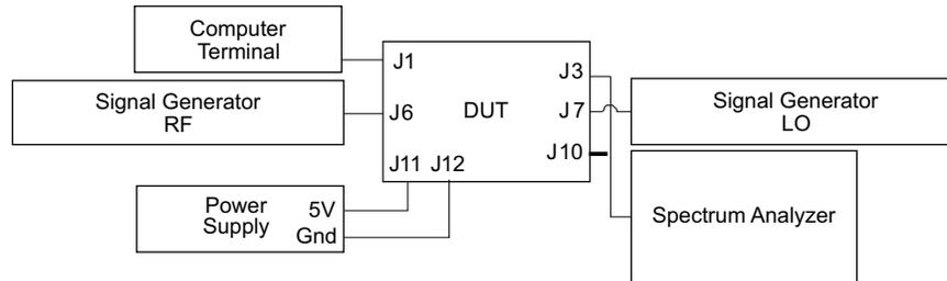
**Figure 3. Test Setup Block Diagram**
