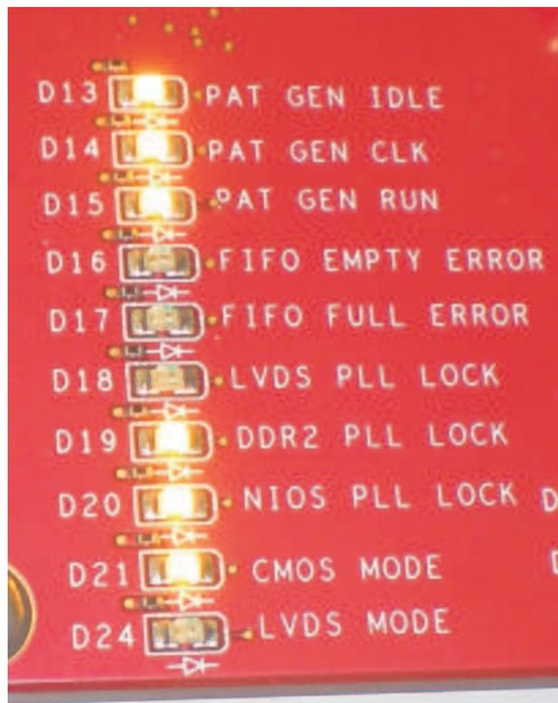
**Figure 16. TSW3100 LED Status With Test Pattern Running**
