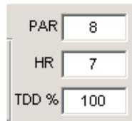
For this example, the PAR and Headroom settings were kept as the default values of 8 dB and 7 dB. The PAR and HR settings can be adjusted later after the signal is loaded by selecting the PAR/HR button.
