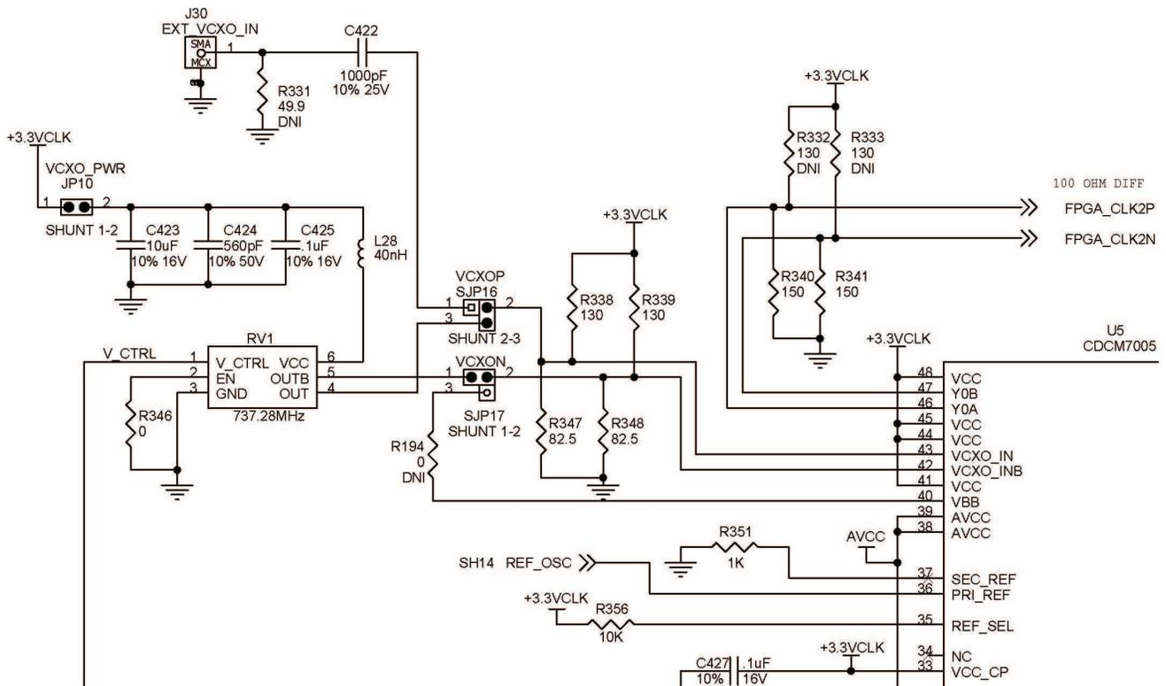
Remove shunt on SJP16 and SJP17. Add shunt on SJP16 pins 1-2 and shunt SJP17 pins 2-3. An 8-dBm CW can be injected into the J30 MCX connector as the external clock. The CDCM7005 in this case only acts as a buffer and clock divider.
