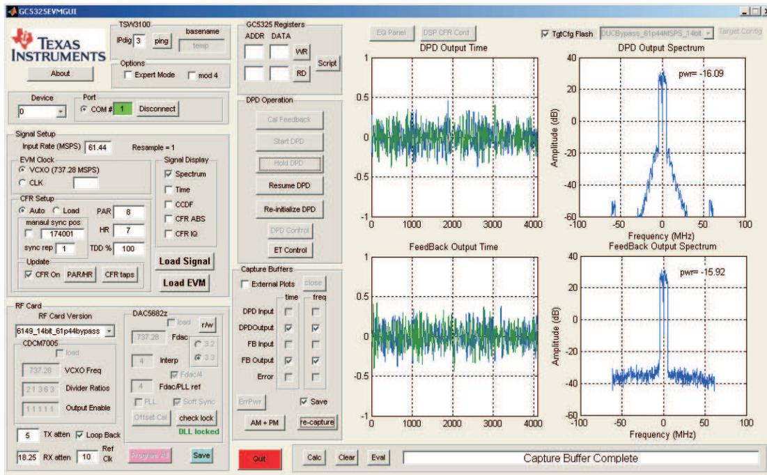
**Figure 19. DPD Results From Internal PA for Channel 0**
