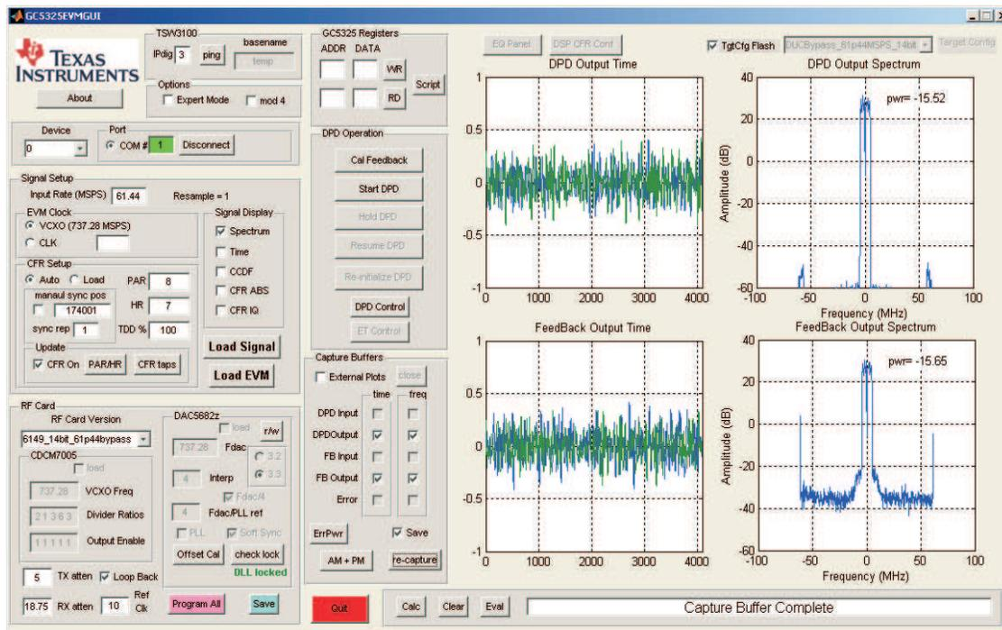
**Figure 18. Loopback Results Using GC5325 Internal Capture Buffers**
