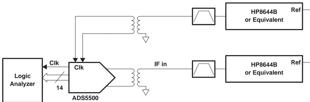
Figure 12. ADC Evaluation Test Set Up (Baseline)
