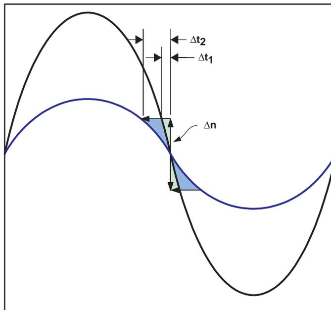
**Figure 6. Thermal Noise Effect for Different Amplitude Sinusoids**
