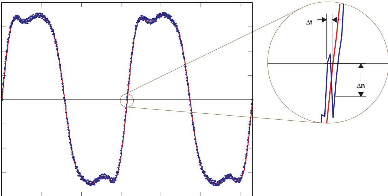
**Figure 4. Thermal Noise Component Causing Sampling Error**
