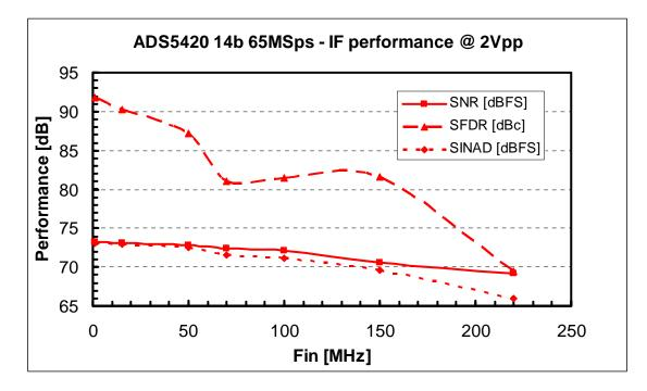
Fig. 10. fiv sweep at 65MSps sampling rate on TI's ADS5420 14 bit 65MSps A-to-D converter for wireless infrastructure applications
