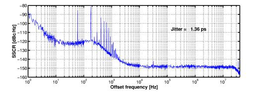
Fig. 9. SSCR vs. fn offset frequency profile of the external source at 30MHz, as obtained from the Aeroflex PN9000 phase noise analyzer
