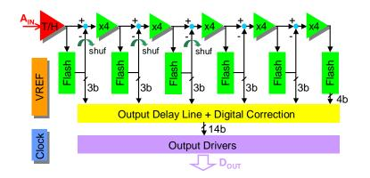
Fig. 8. Pipelined converter architecture (2.5 bit per stage), with integrated internal references and on-chip clock driver
