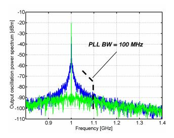
Fig. 2. Matlab simulated signals spectra in detail. The upper spectrum pertains to oscillators showing white frequency noise (free running VCO), the lower one by highpass-filtered frequency noise (typical of PLL)
