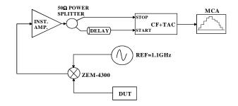
Fig. 4. Block diagram of the lab setup. A low-noise instrumentation amplifier can provide for image rejection, whereas the coaxial stub is used to synchronize the operation of the zero-crossing detector [3]
