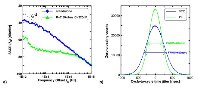
Fig. 5. a) Experimental SSCR curves for the LC-tuned VCO and PLL built around it. The discrepancy with the pure 1/f<sup>2</sup> trend of the VCO plot is due to a residual PLL action. b) Statistical distributions of the period duration as collected at the MCA of the setup in Fig. 4
