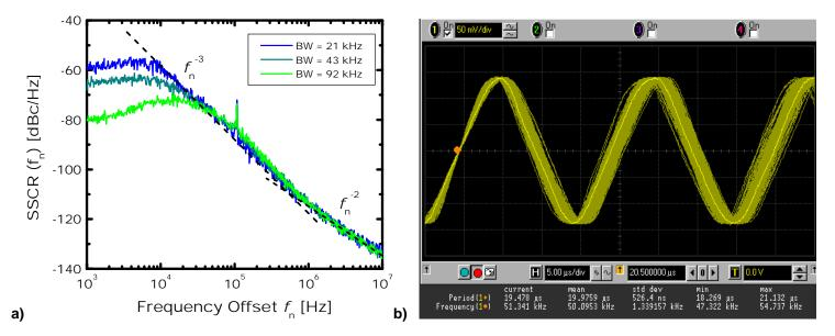
Fig. 7. a) Experimental SSCR plots for the CMOS PLL frequency synthesizer operated with different bandwidths. b) The jittering zerocrossings of the PLL output, as captured with an Agilent Infinitum™ oscilloscope
