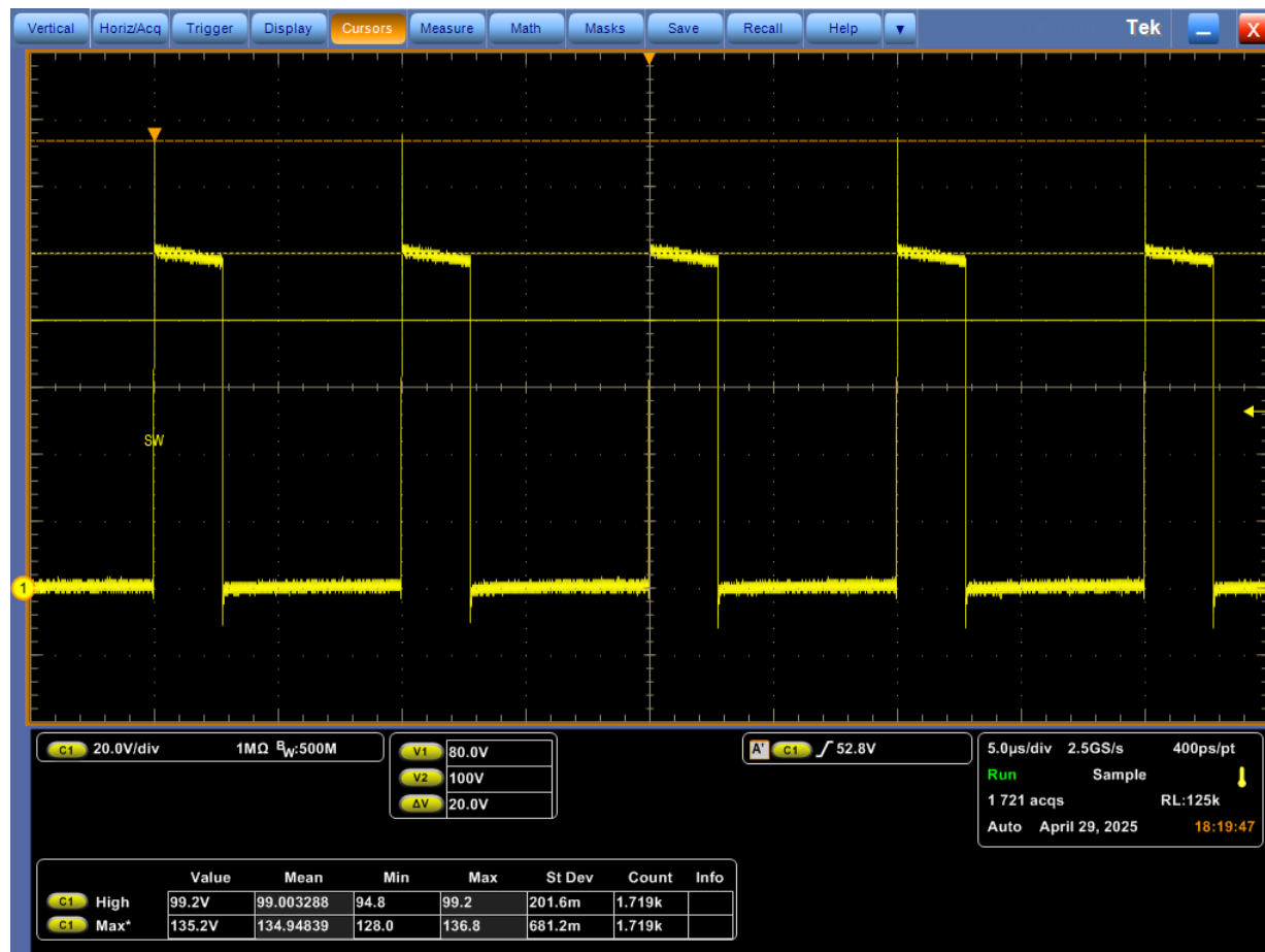
Figure 3-3. Phase Node Voltage
