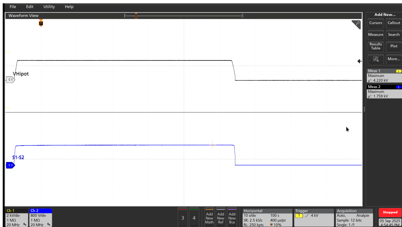
Figure 3-3. Secondary Sense (S1) and Voltage Sense (S2) Test Points at HV = 4300V
