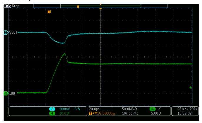
Figure 3-4. Transient Response to Load Step 500mA to 24A
