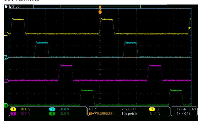
Figure 3-1. Quadrature Switch Nodes
