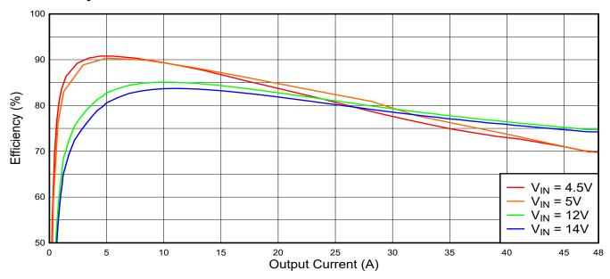
Figure 3-7. Efficiency FSW = 500kHz
