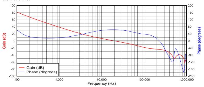
Figure 3-6. Frequency Response IOUT = 24A
