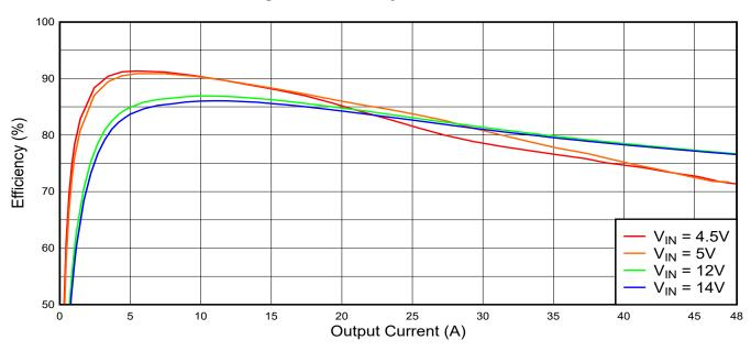
Figure 3-8. Efficiency FSW = 200kHz
