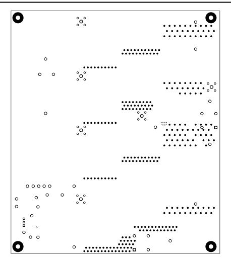
Figure 4-15. Solder Mask (Bottom View)
