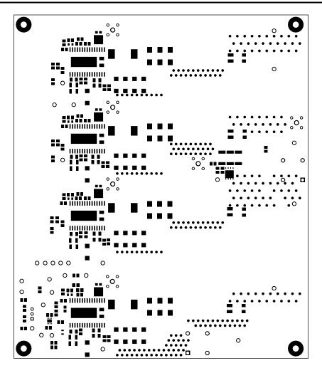
Figure 4-6. Solder Mask (Top View)
