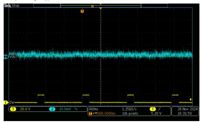
Figure 3-2. Output Voltage Ripple
