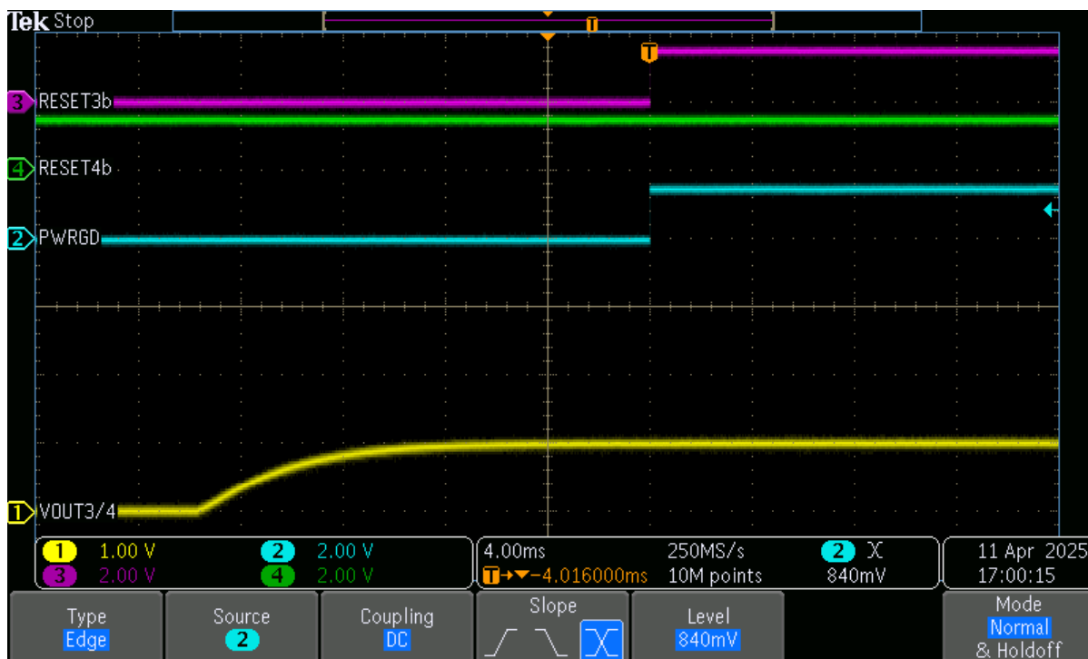
Figure 3-5. Channel 3/4 Enter Regulation with DLY_TMR=619kOhms
