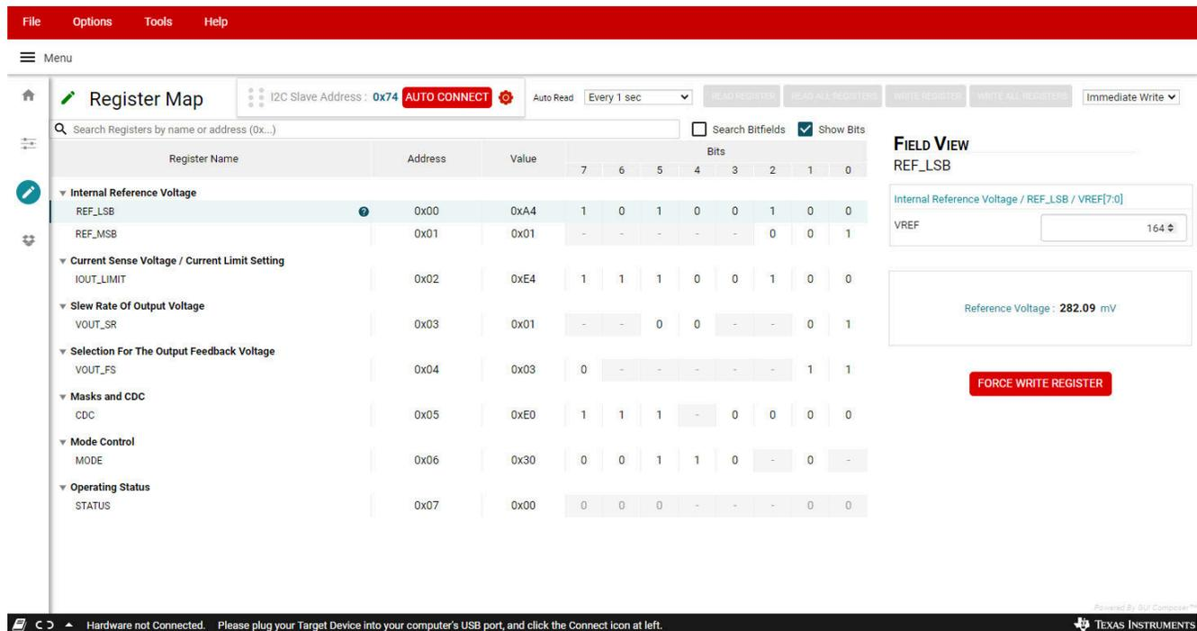
**Figure 3-7. GUI Register Map Screen**
