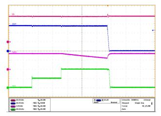
Figure 3-8. Persistent Overload Performance of TPS1685 eFuse ( $V_{IN}$  = 54V,  $C_{ITIMER}$  = 27nF,  $C_{OUT}$  = 1mF,  $R_{IMON}$  = 1.1k $\Omega$  ( $I_{OCP}$  = 50A),  $R_{IREF}$  = 40.2k $\Omega$  ( $V_{REF}$  = 1V), and  $I_{OUT}$  Ramped from 40A for 10ms to 80A for 20ms)
