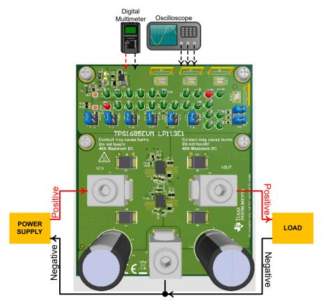
Figure 3-1. TPS1685EVM Setup with Test Equipment
