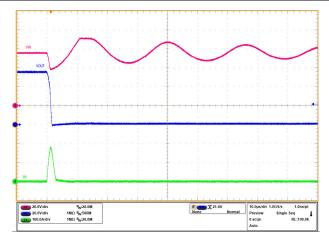
Figure 3-10. Output Hot Short Response (zoomed in) in TPS1685EVM ( $V_{IN}$  = 54V,  $R_{IMON}$  = 1.1k $\Omega$ ,  $R_{IREF}$  = 40.2k $\Omega$ , R<sub>SFT</sub> = 150k $\Omega$ , and C<sub>OUT</sub> = 1mF)
