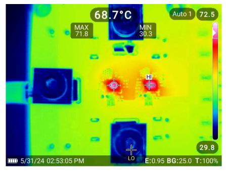
Figure 3-13. Thermal Performance of TPS1685EVM ( $V_{IN}$  = 54V,  $I_{OUT}$  = 40A,  $T_A$  = 30°C, and No External Air Flow)
