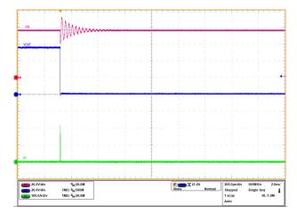
Figure 3-9. Output Hot Short Response (zoomed out) in TPS1685EVM ( $V_{IN}$  = 54V,  $R_{IMON}$  = 1.1k $\Omega$ ,  $R_{IREF}$  = 40.2k $\Omega$ ,  $R_{SFT}$  = 150k $\Omega$ , and  $C_{OUT}$  = 1mF)
