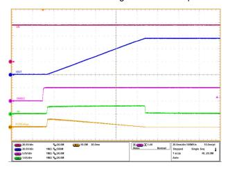
Figure 3-3. TPS1685 eFuse Start-up Profile with ENABLE ( $V_{IN}$  = 54V, EN Stepped Up from 0V to 5V,  $C_{OUT}$  = 1mF, and  $C_{DVDT}$  = 82nF)
