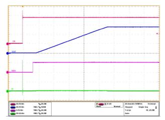
Figure 3-2. TPS1685 eFuse Hot Plug Profile ( $V_{IN}$  Stepped Up from 0V to 54V,  $C_{OUT} = 1$ mF, and  $C_{DVDT} = 82$ nF)
