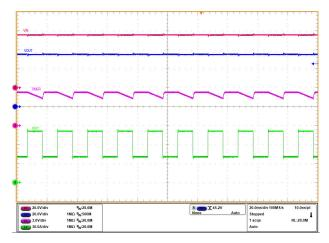
Figure 3-7. Transient Overload Performance of TPS1685 eFuse ( $V_{IN}$  = 54V,  $C_{ITIMER}$  = 27nF,  $C_{OUT}$  = 1mF,  $R_{IMON}$  = 1.1k $\Omega$  ( $I_{OCP}$  = 50A),  $R_{IREF}$  = 40.2k $\Omega$  ( $V_{REF}$  = 1V), and  $I_{OUT}$  Ramped from 40A for 10ms to 80A for 10ms)
