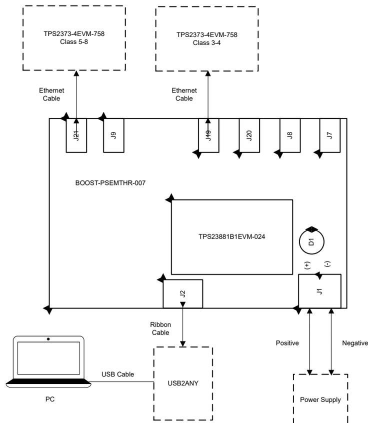
**Figure 2-1. Basic Setup Using USB2ANY**
