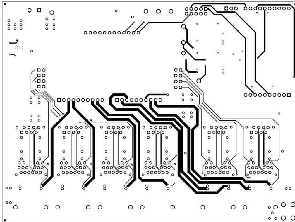
Figure 4-8. BOOST-PSEMTHR-007 (Motherboard) Bottom Side Routing
