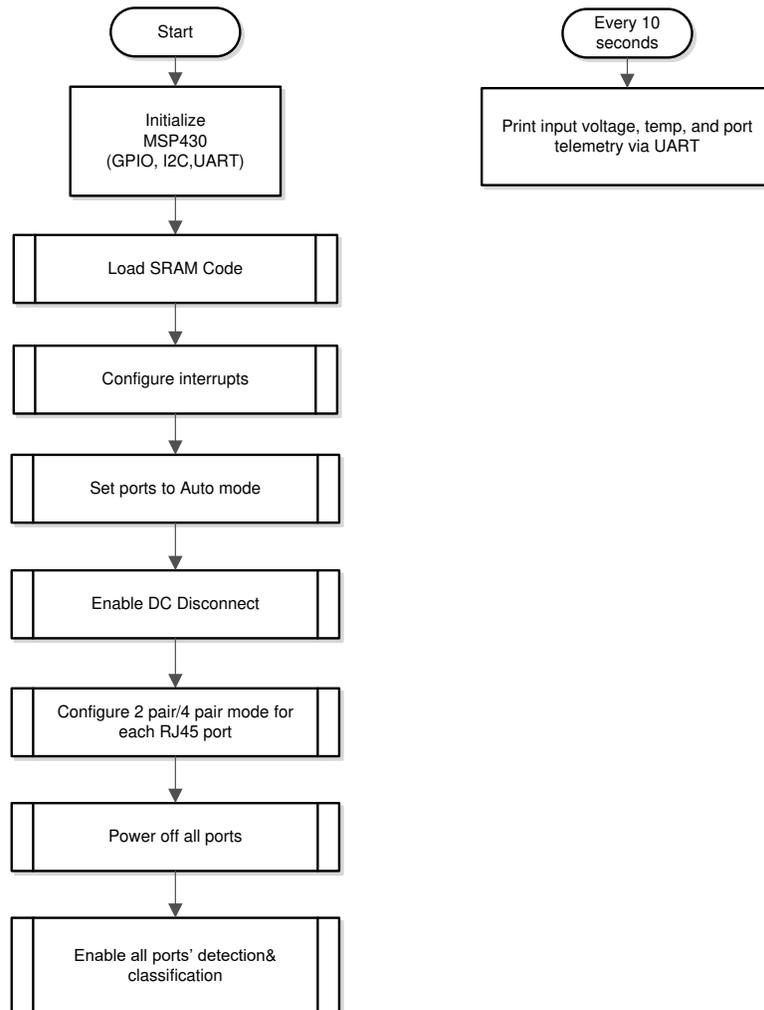
**Figure 3-8. Auto Mode System Software Structure**
