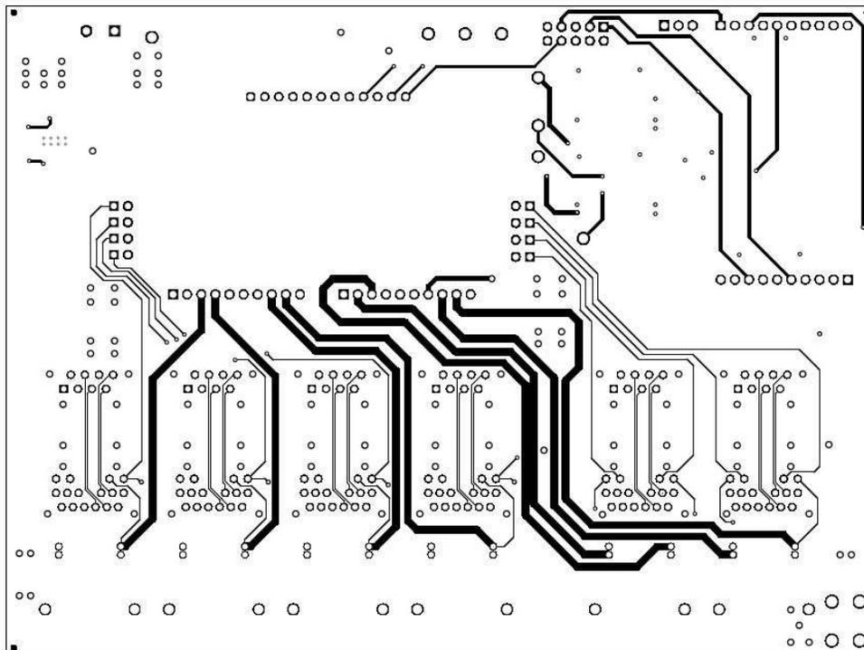
**Figure 4-5. BOOST-PSEMTHR-007 (Motherboard) Top Side Routing**
