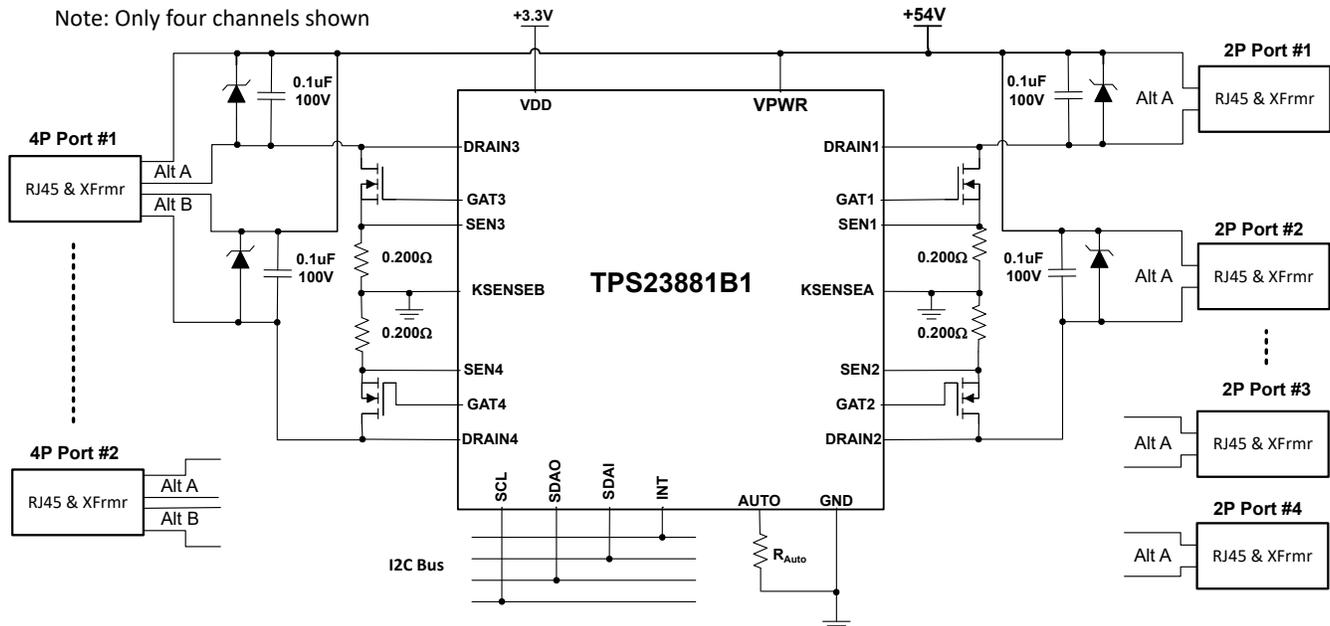
Figure 1-1. TPS23881B1 Device Block Diagram
