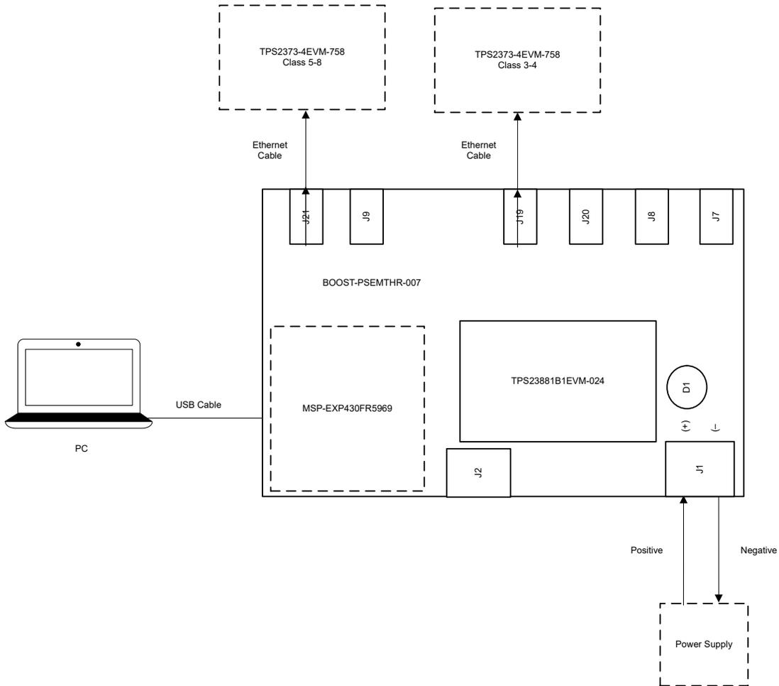
**Figure 2-2. Advanced Setup Using LaunchPad**
