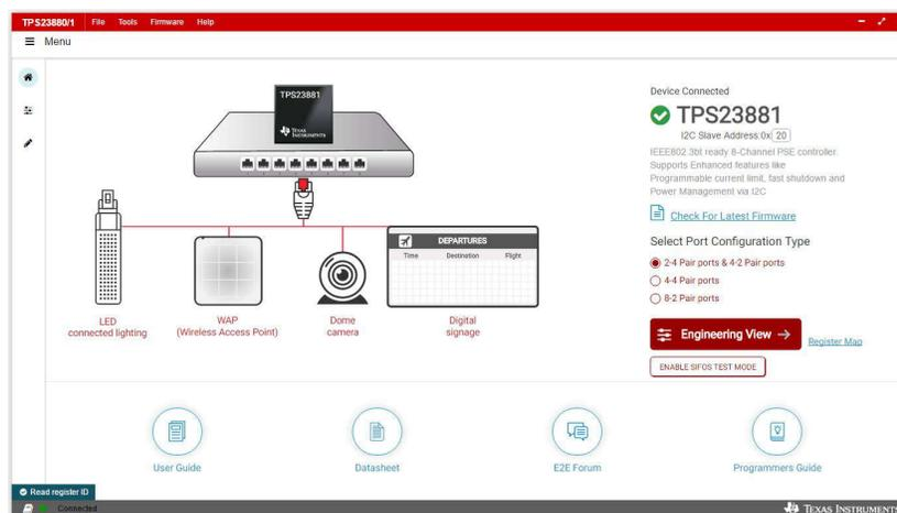
**Figure 3-1. TPS23881B1EVM GUI Start-up Window**
