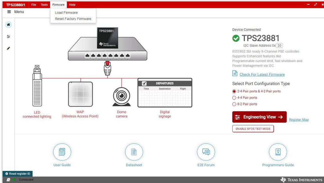
Figure 3-2. TPS23881B1EVM GUI Load Firmware 1
