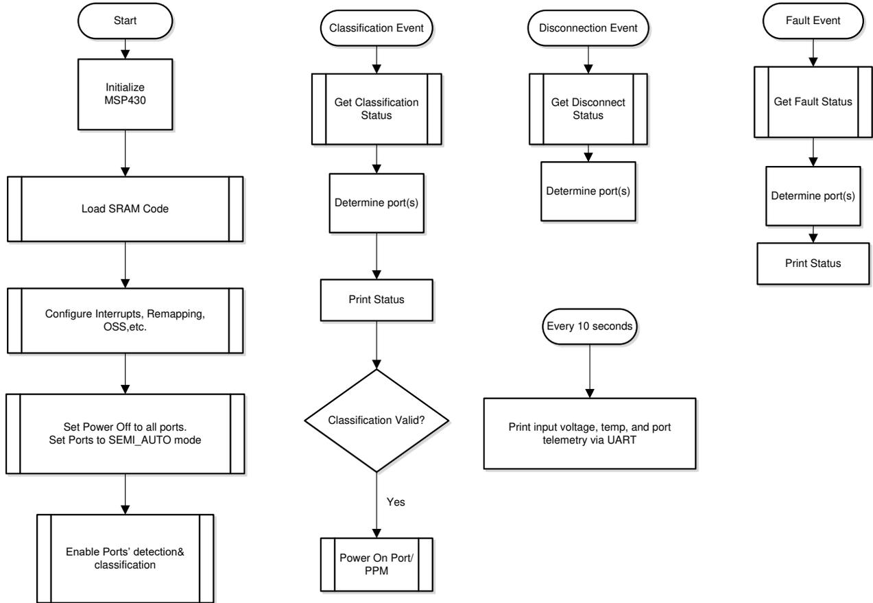
**Figure 3-9. Semi Auto Mode System Software Structure**
