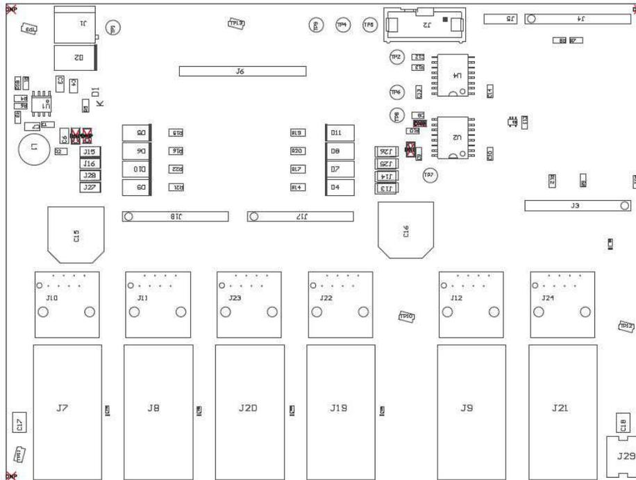
**Figure 4-4. BOOST-PSEMTHR-007 (Motherboard) Top Side Assembly**
