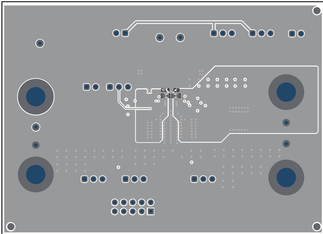
Figure 4-5. TPS55289Q1EVM-011 Bottom-Side Layout
