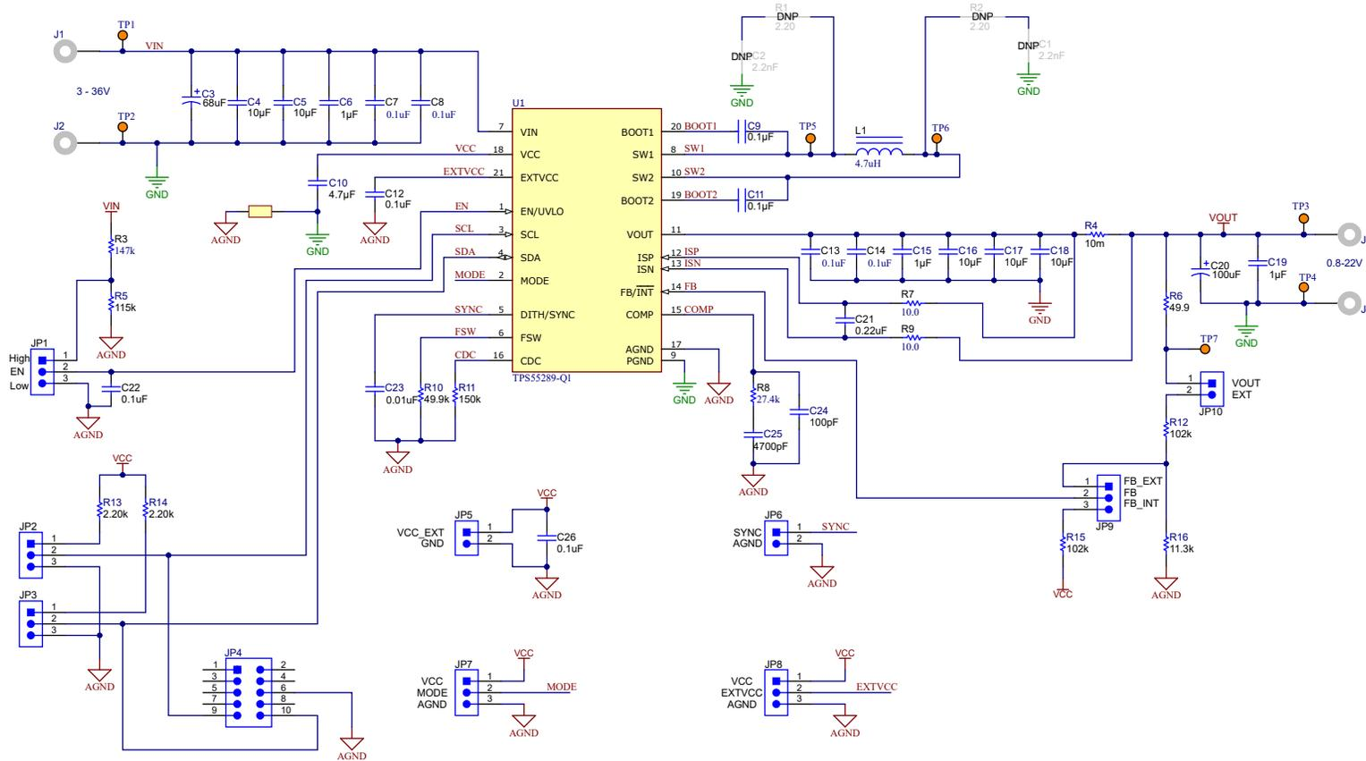
Figure 4-1. TPS55289Q1EVM-011 Schematic
