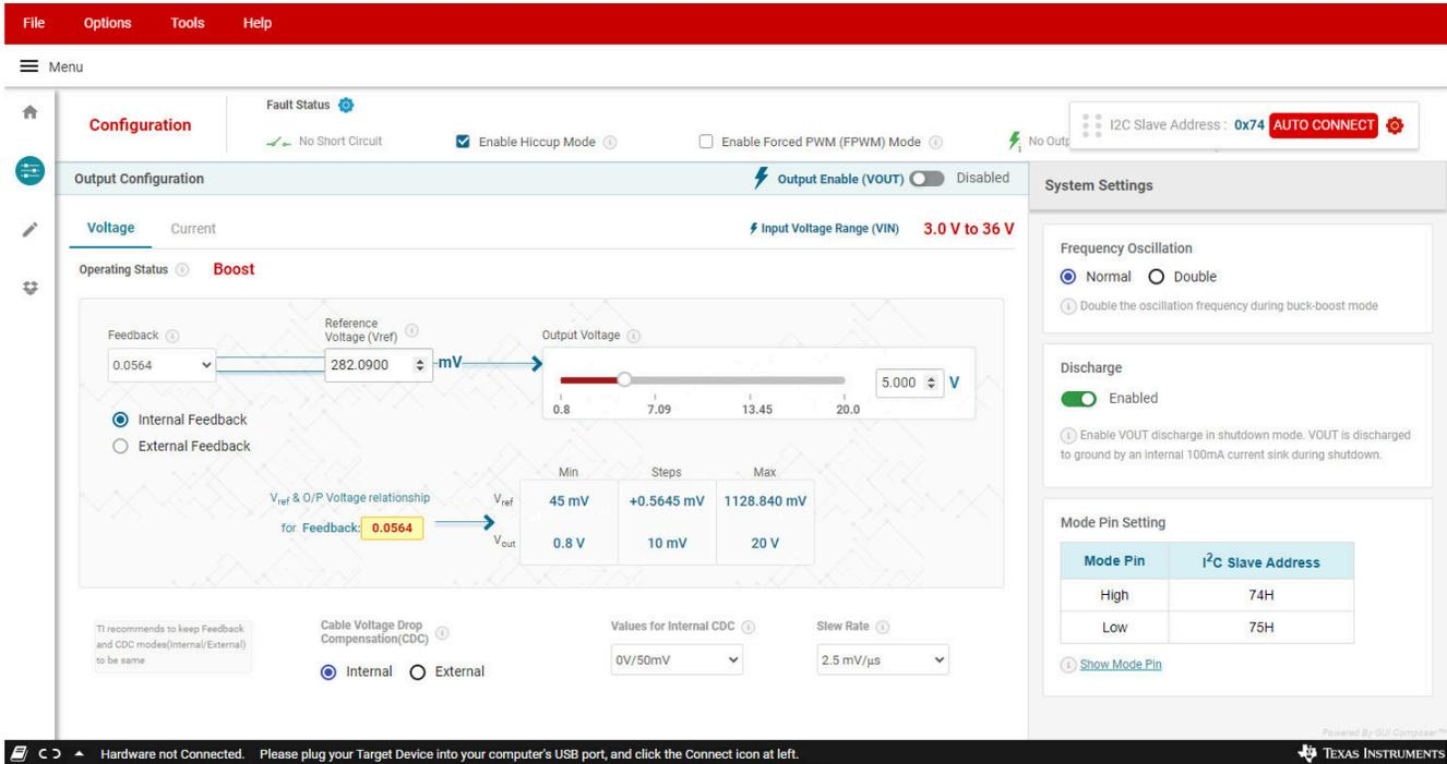
Figure 3-4. GUI User Interface of TPS55289Q1EVM-011
