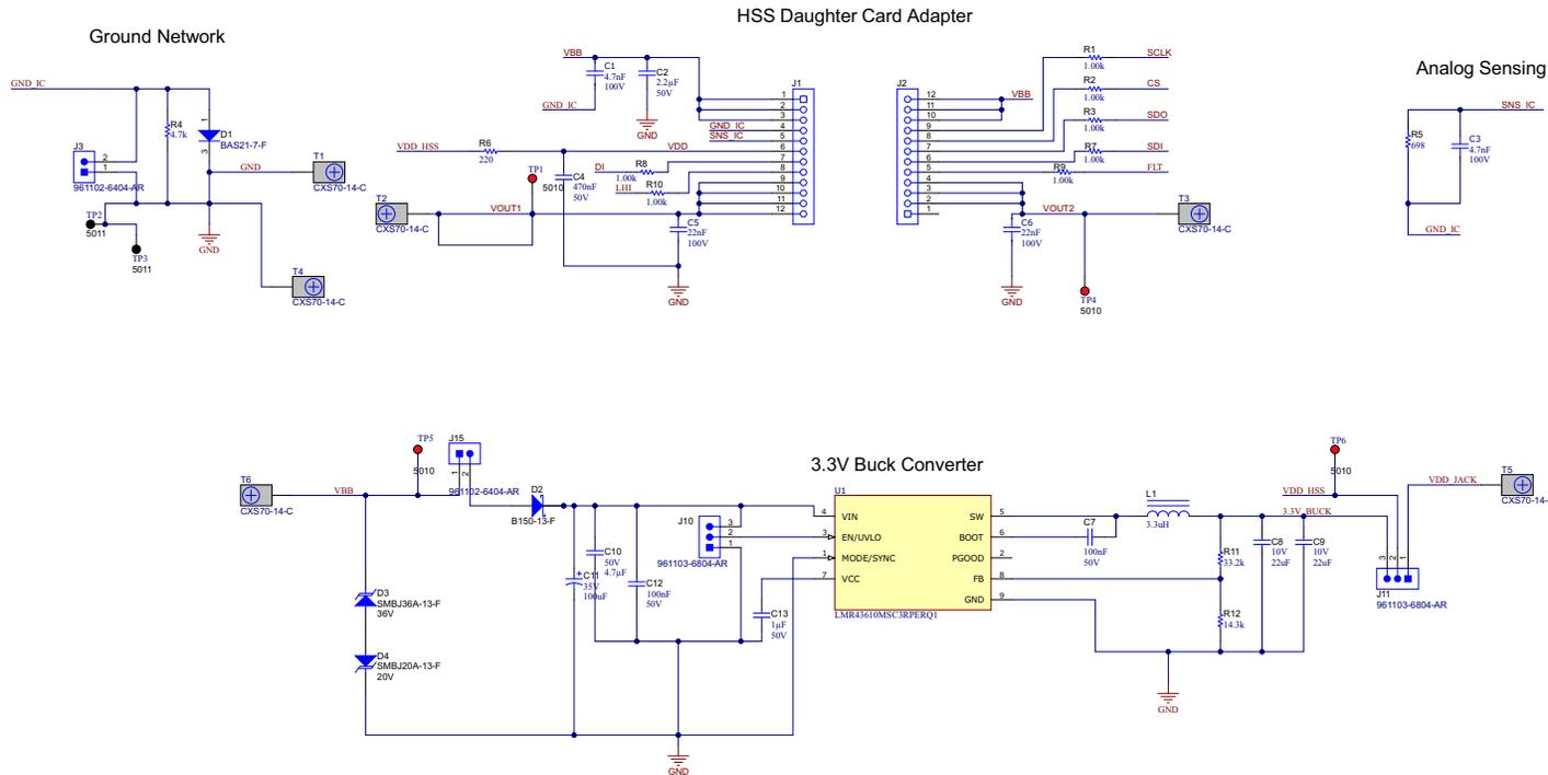
Figure 4-2. Motherboard Schematic - High-Side Switch
