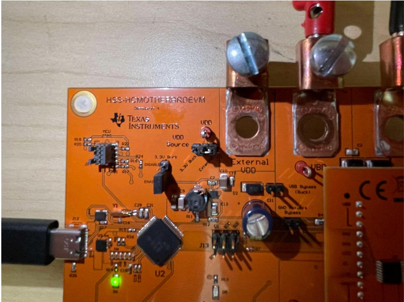
**Figure 2-8. Configured for External VDD**
