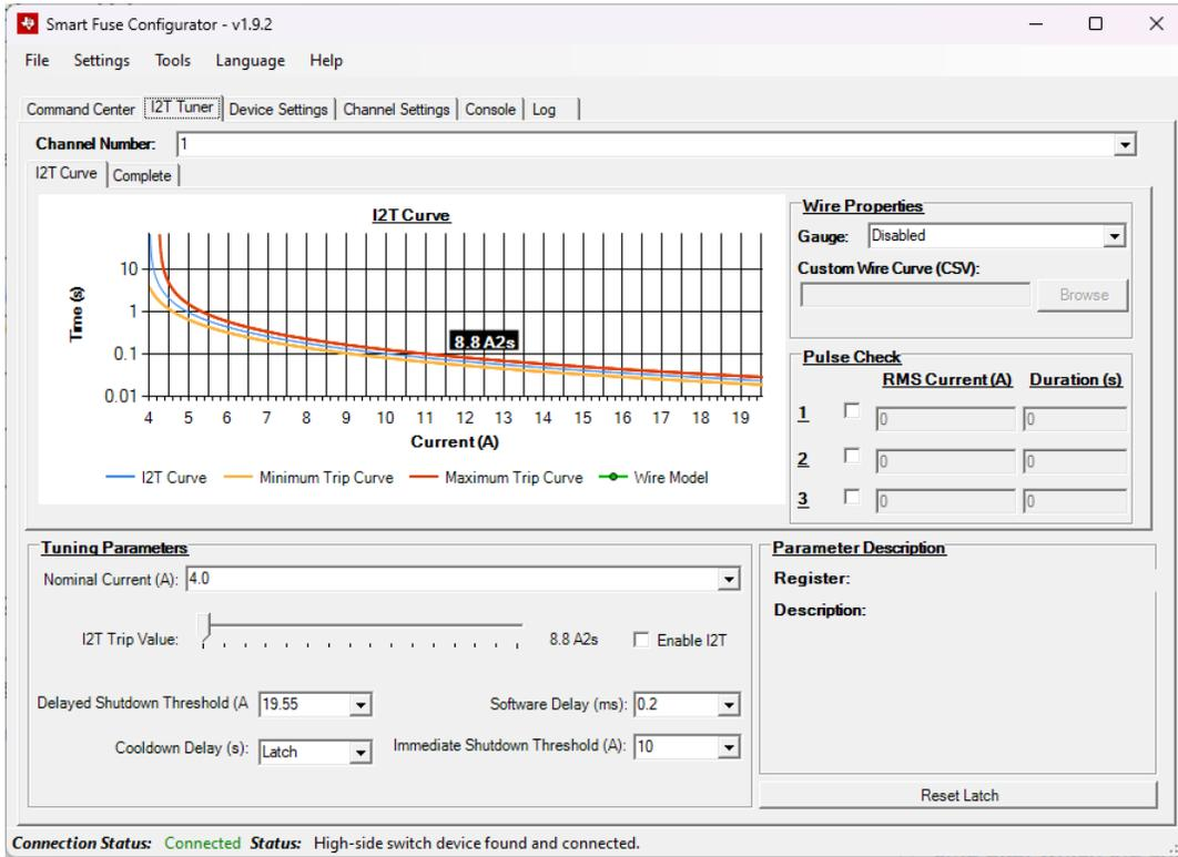
Figure 3-6. I2T Curve Tuner
