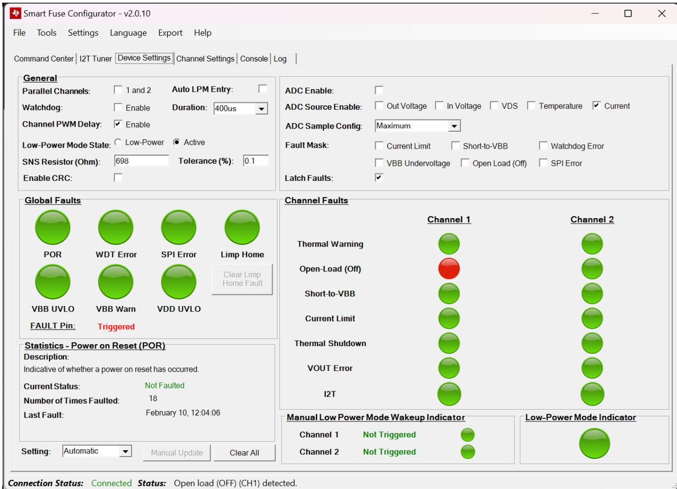
Figure 3-12. Faulted Device View
