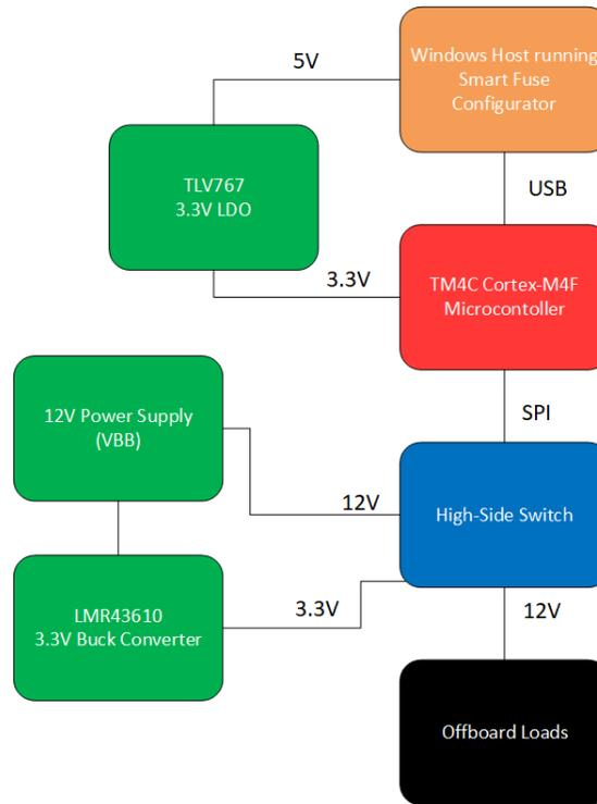
**Figure 1-1. Block Diagram for HSS-HCMOTHERBRDEVM**
