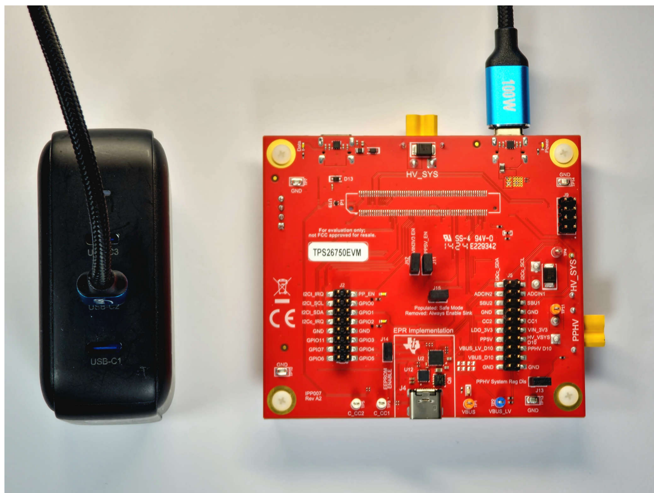
Figure 2-3. Stand Alone Testing Example Hardware Setup
