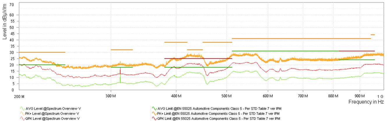
**Figure 5-16. CISPR 25 Radiated Emissions: 200 MHz to 1 GHz, LOG**
