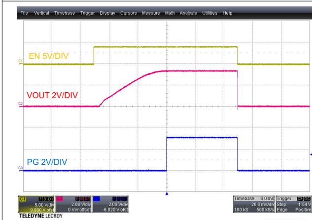
Figure 5-8. Enable ON and OFF
