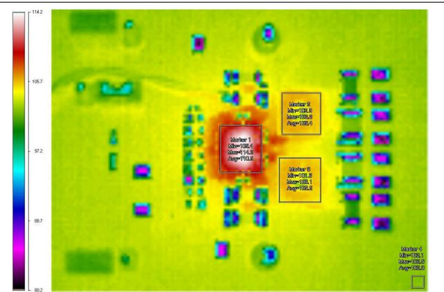
Figure 5-25. Infrared Thermal Image: VIN = 12 V, T<sub>AMB</sub> = 85°C, 200LFM, I<sub>OUT</sub> = 6 A
