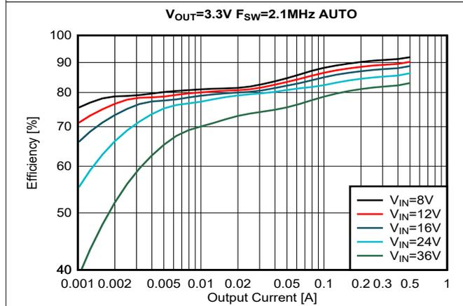
Figure 5-3. Efficiency,  $V_{OUT} = 3.3\text{ V}$ , AUTO Mode
