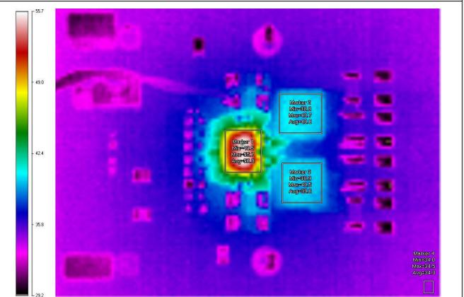
Figure 5-21. Infrared Thermal Image: VIN = 12 V, T<sub>AMB</sub> = 25°C, 200LFM, IOUT = 10 A
