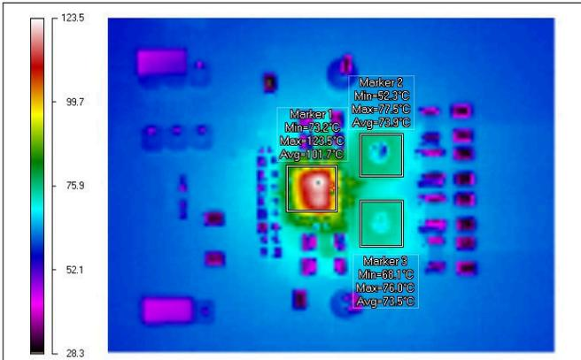
Figure 5-18. Infrared Thermal Image: VIN = 12 V, IOUT = 12 A
