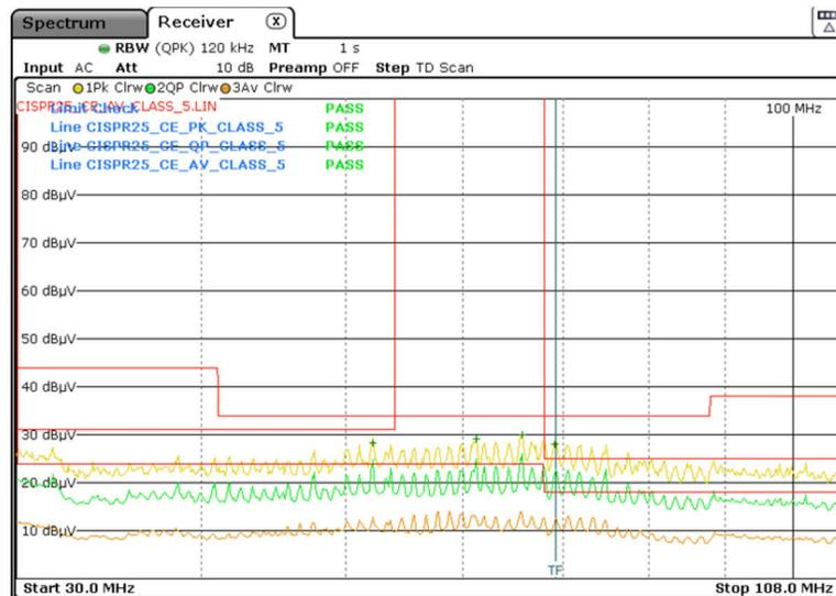
Figure 5-13. CISPR 25 Conducted Emissions: 30 MHz to 108 MHz
