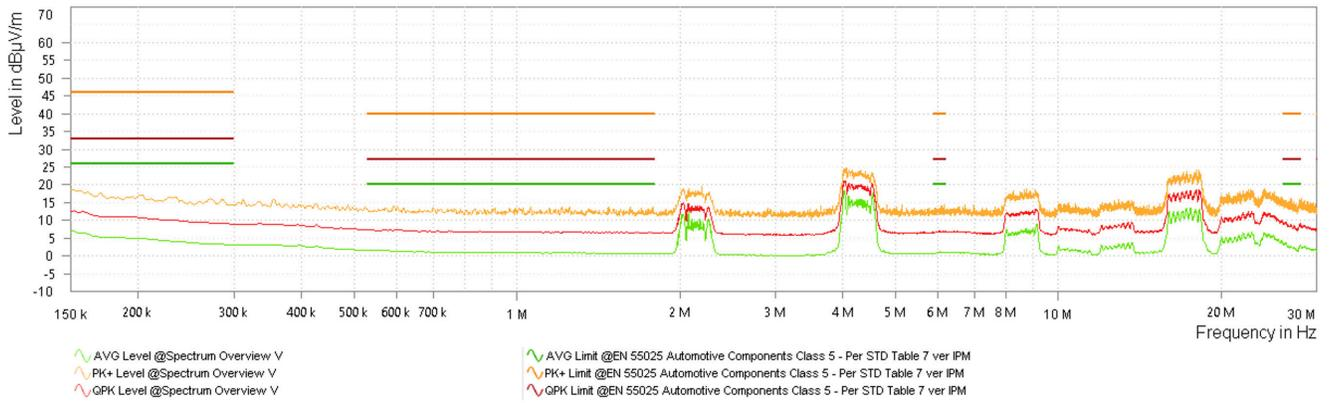
**Figure 5-14. CISPR 25 Radiated Emissions: 150 kHz to 30 MHz, MONOPOLE**
