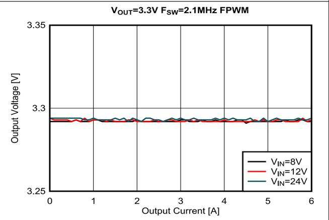
Figure 5-4. Load Regulation,  $V_{OUT} = 3.3\text{ V}$ , FPWM Mode
