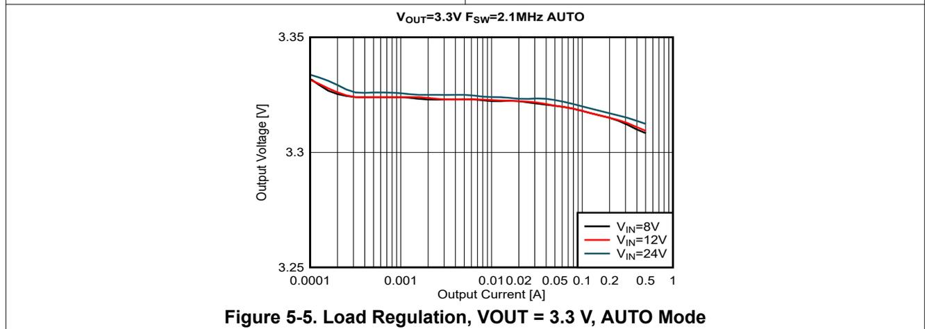
Figure 5-5. Load Regulation,  $V_{OUT} = 3.3\text{ V}$ , AUTO Mode
