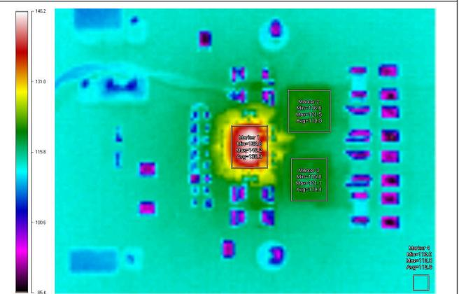
Figure 5-23. Infrared Thermal Image: VIN = 12 V, T<sub>AMB</sub> = 85°C, 200LFM, IOUT = 10 A
