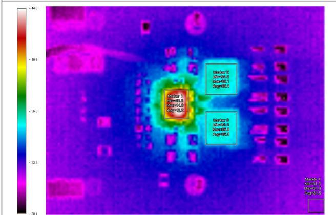
Figure 5-22. Infrared Thermal Image: VIN = 12 V, T<sub>AMB</sub> = 25°C, 200LFM, IOUT = 8 A
