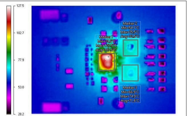
Figure 5-19. Infrared Thermal Image: VIN = 24 V, IOUT = 10 A
