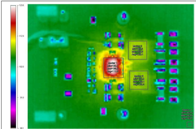
Figure 5-24. Infrared Thermal Image: VIN = 12 V, T<sub>AMB</sub> = 85°C, 200LFM, I<sub>OUT</sub> = 8 A
