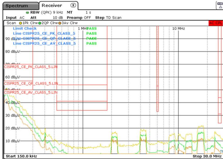
Figure 5-12. CISPR 25 Conducted Emissions: 150 kHz to 30 MHz
