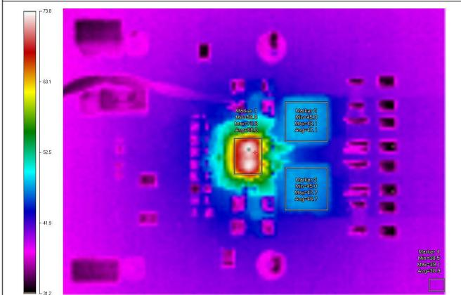
Figure 5-20. Infrared Thermal Image: VIN = 12 V, T<sub>AMB</sub> = 25°C, 200LFM, IOUT = 12 A
