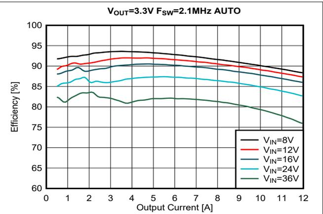
Figure 5-2. Efficiency,  $V_{OUT} = 3.3\text{ V}$ , AUTO Mode
