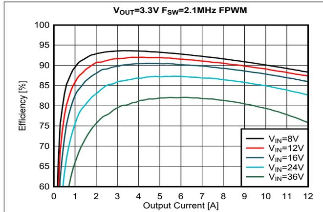
Figure 5-1. Efficiency,  $V_{OUT} = 3.3\text{ V}$ , FPWM Mode
