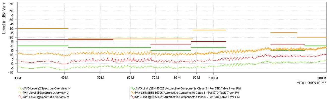
**Figure 5-15. CISPR 25 Radiated Emissions: 30 MHz to 200 MHz, BICON**
