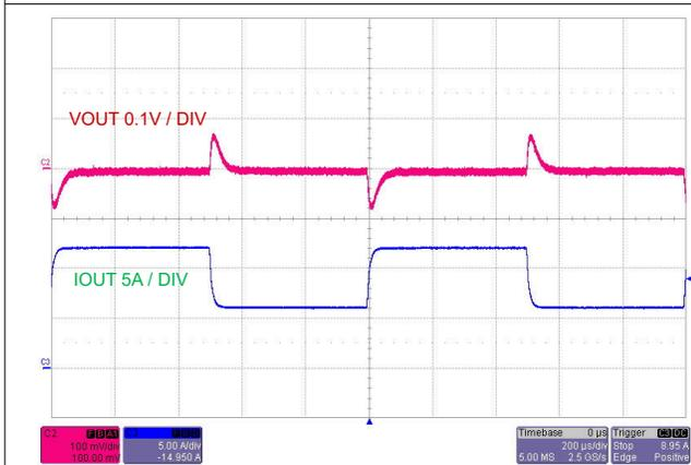
Figure 5-10. Load Transient, 6 A to 12 A
