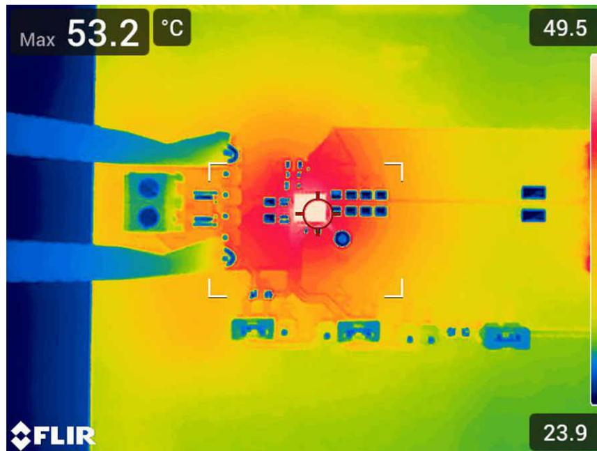
Figure 4-2. Thermal Performance (TPSM8286AA0HEVM,  $V_{IN} = 5\text{ V}$ ,  $V_{OUT} = 1.2\text{ V}$ ,  $I_{OUT} = 6\text{ A}$ )
