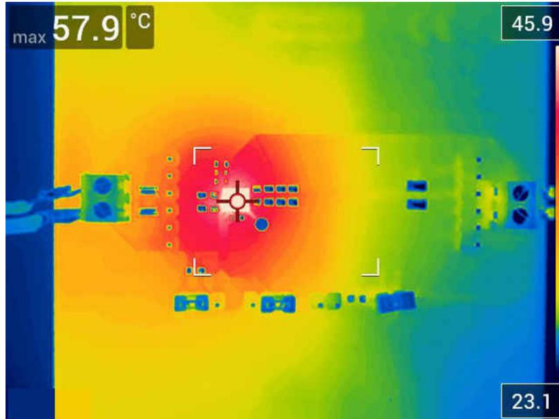
Figure 4-1. Thermal Performance (TPSM8286AA0SEVM,  $V_{IN} = 5\text{ V}$ ,  $V_{OUT} = 1.2\text{ V}$ ,  $I_{OUT} = 6\text{ A}$ )
