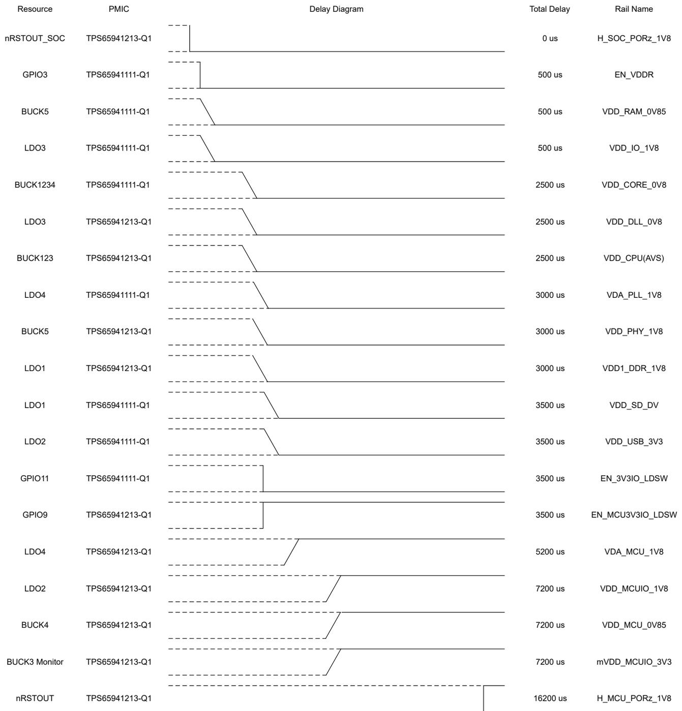
**Figure 6-10. TO\_MCU Sequence with I2C\_7 low in both PMICs**
