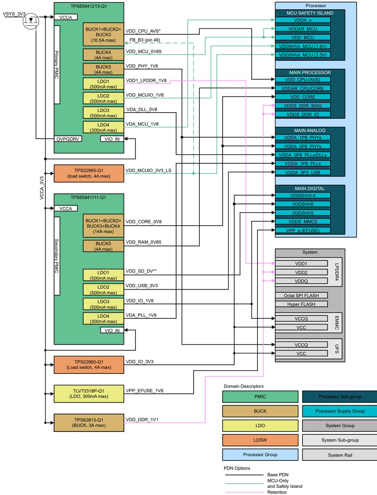
Figure 3-1. Power Connections
