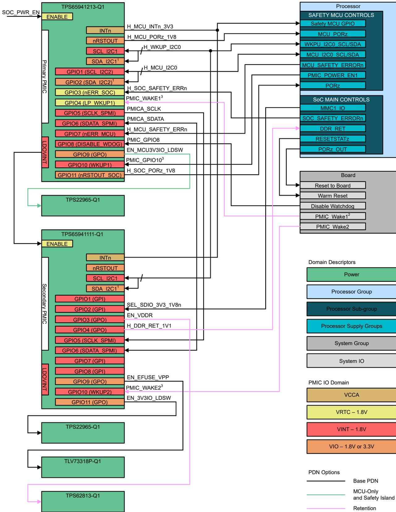
Figure 3-2. TPS6594-Q1 Digital Connections
