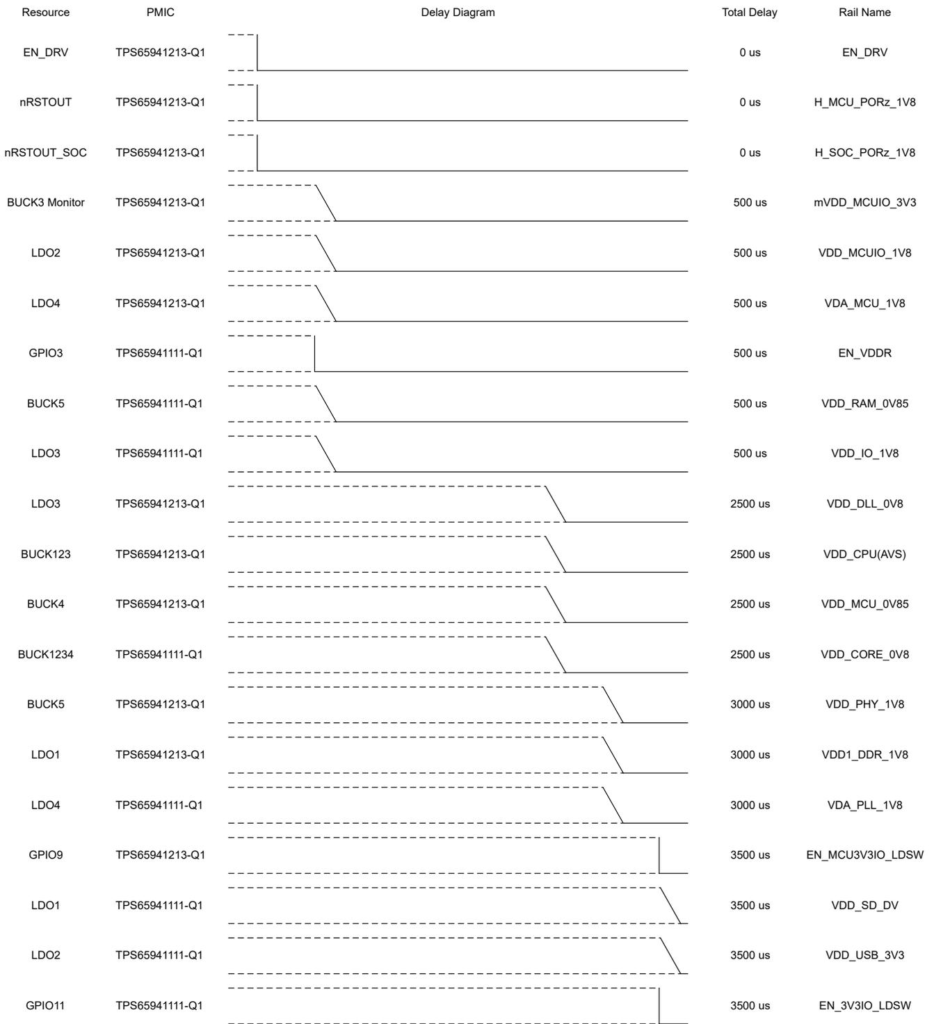
**Figure 6-12. TO\_RETENTION when I2C\_7 is low in both PMICs**
