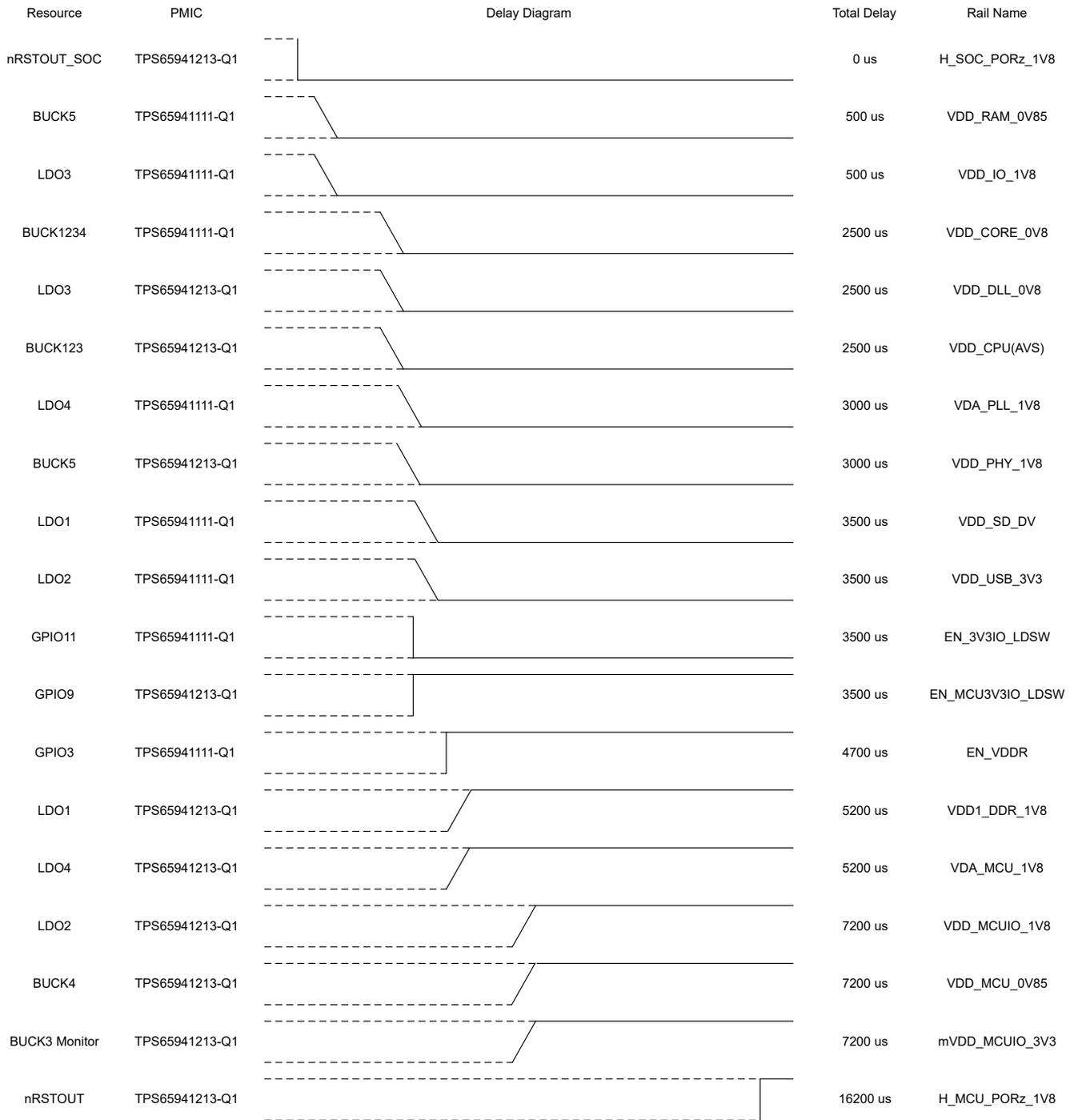
Figure 6-9. TO\_MCU with I2C\_7 high in both PMICs
