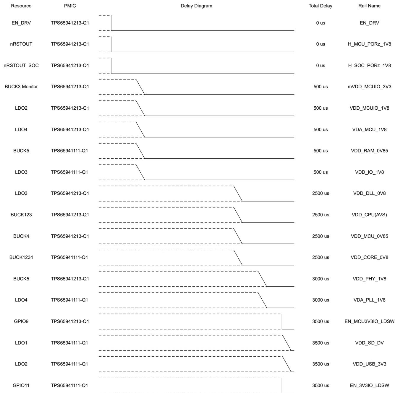
**Figure 6-13. TO\_RETENTION when I2C\_7 is high in both PMICs**
