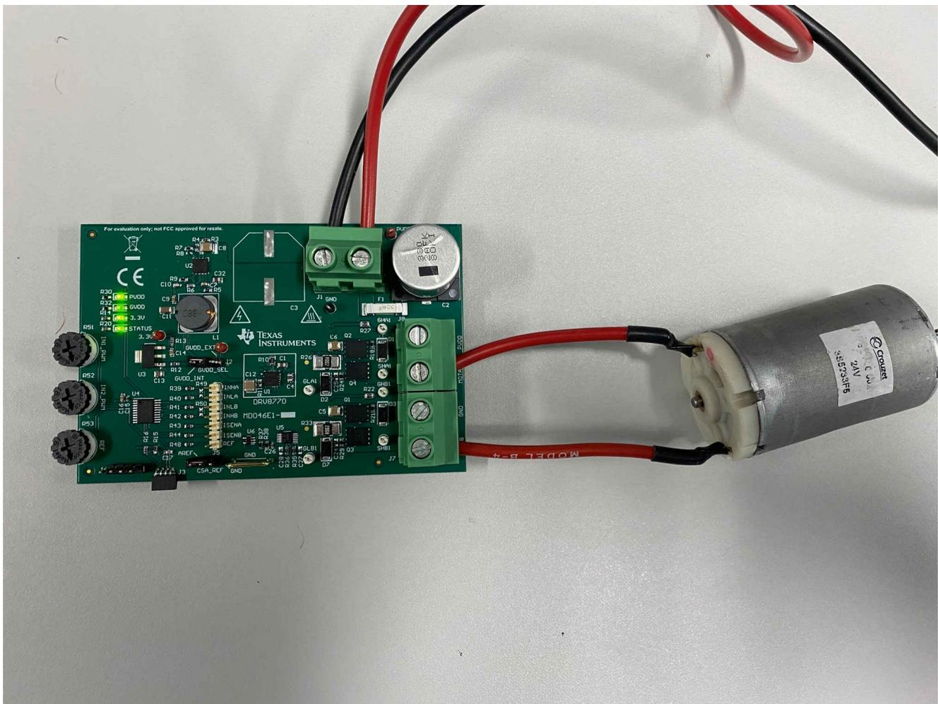
**Figure 3-1. EVM Power Supply and Motor Connections**
