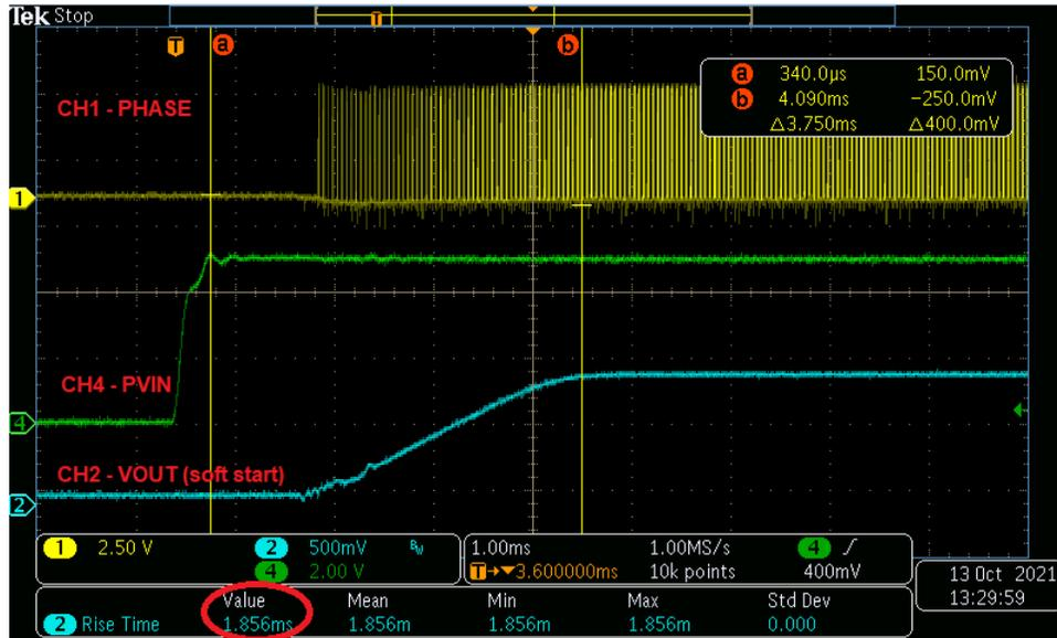
Figure 4-3. Output Soft Start Voltage, VIN = 5V, VOUT = 1V, IOU = 18A
