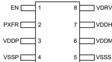
Figure 1-3. TPSI3050-Q1, TPSI3050S-Q1 DWZ Package 8-Pin SOIC Top View
