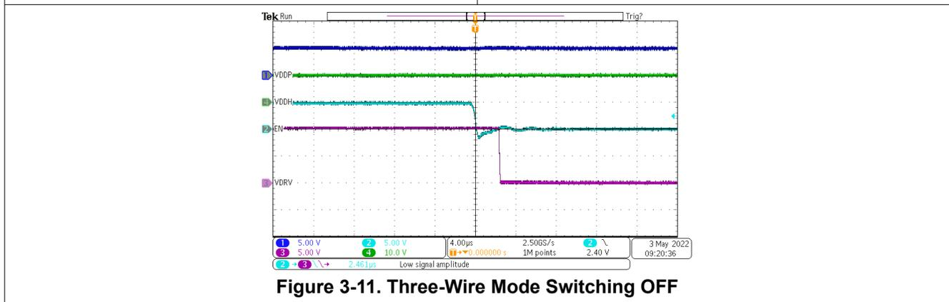
**Figure 3-11. Three-Wire Mode Switching OFF**
