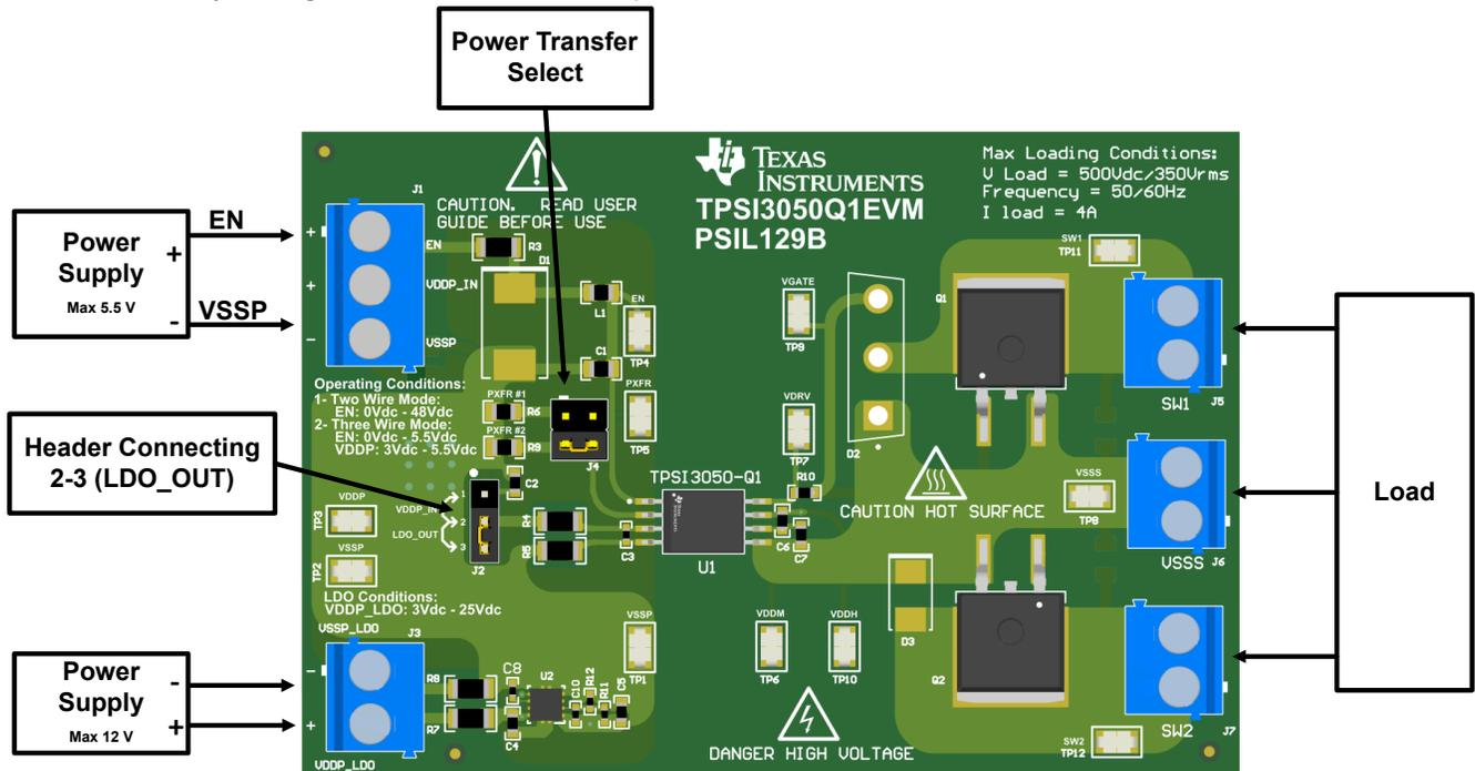
**Figure 3-8. Three-Wire Mode VDDP Supply Through 5-V LDO**
