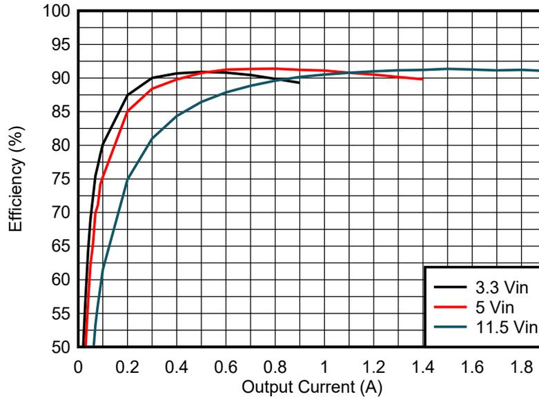
Figure 3-1. Efficiency for -5 V Output with 1MHz f<sub>sw</sub>
