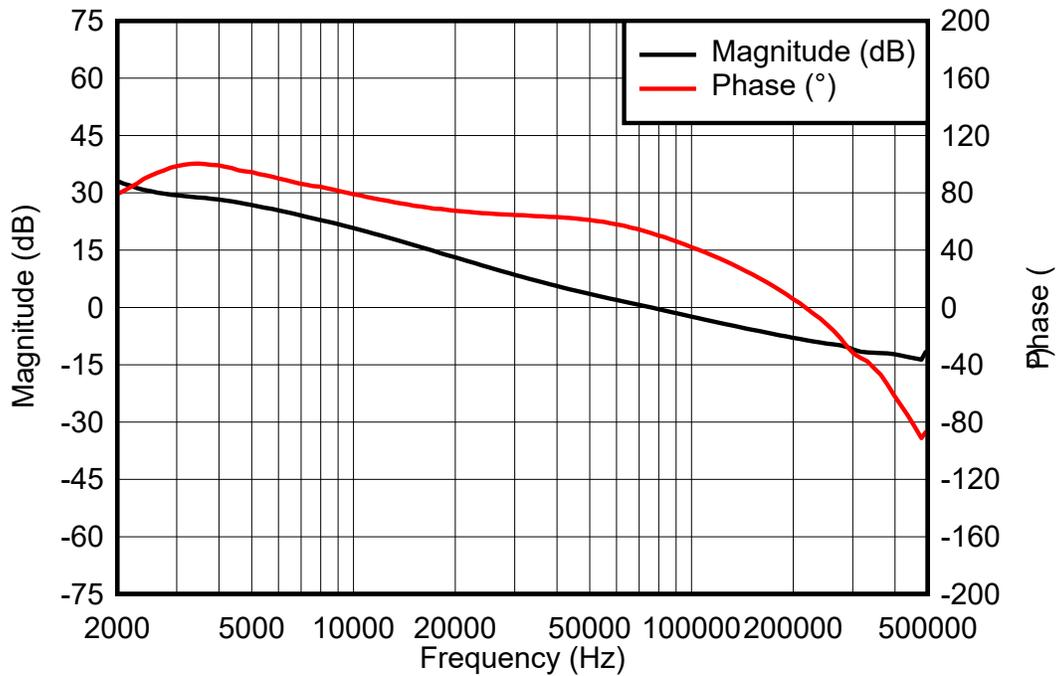
**Figure 3-6. Loop Response Measurement ( $V_{IN} = 5\text{ V}$ ,  $V_{OUT} = -5\text{ V}$ ,  $I_{OUT} = 1000\text{ mA}$ , Ferrite Bead Removed)**
