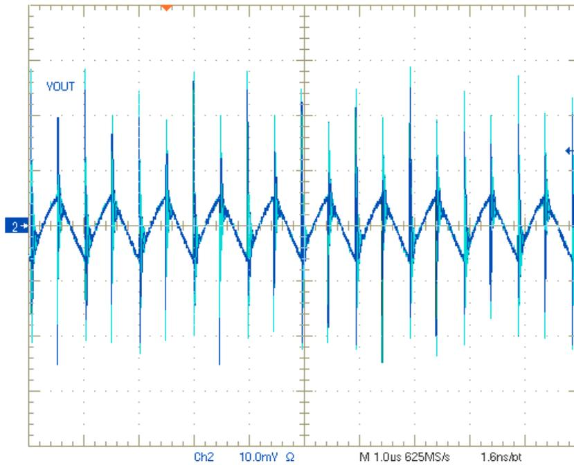
$V_{IN} = 5\text{ V}$ ,  $V_{OUT} = -5\text{ V}$ ,  $I_{OUT} = 1000\text{ mA}$ ,  $FSW = 1\text{ MHz}$ , Full BW, DC Coupling, 50-Ω Termination With DC Blocker
