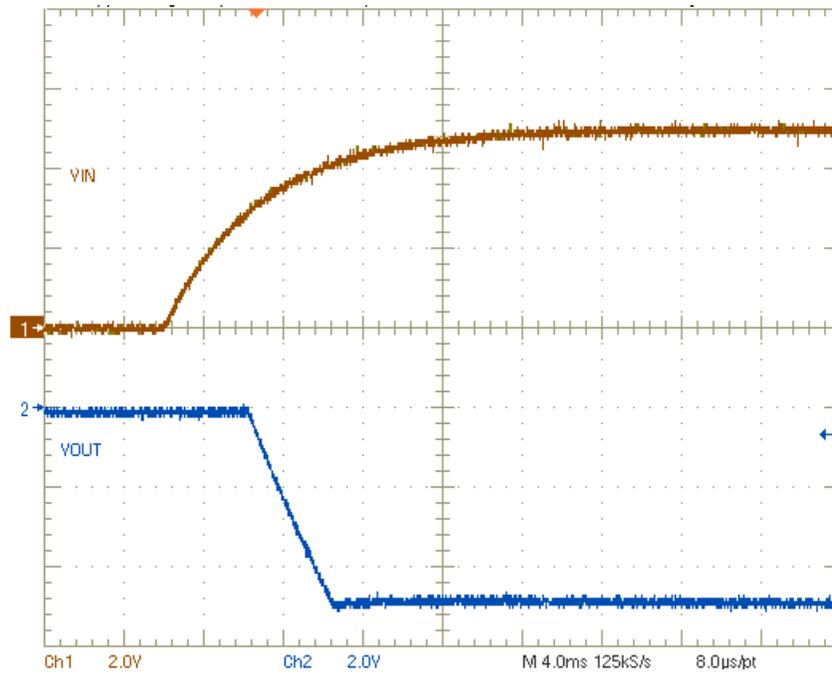
Figure 3-3. Startup with 1A Load
