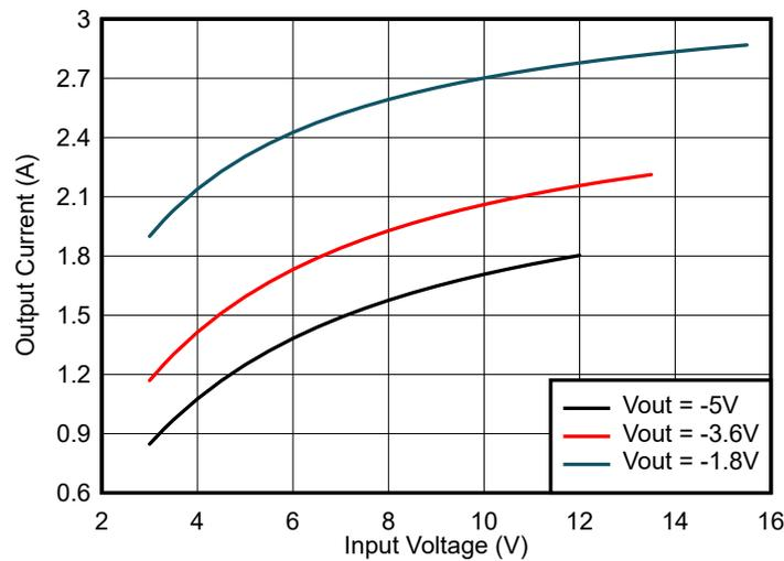
**Figure 1-1. Output Current Limitations by Input Voltage and Output Voltage**
