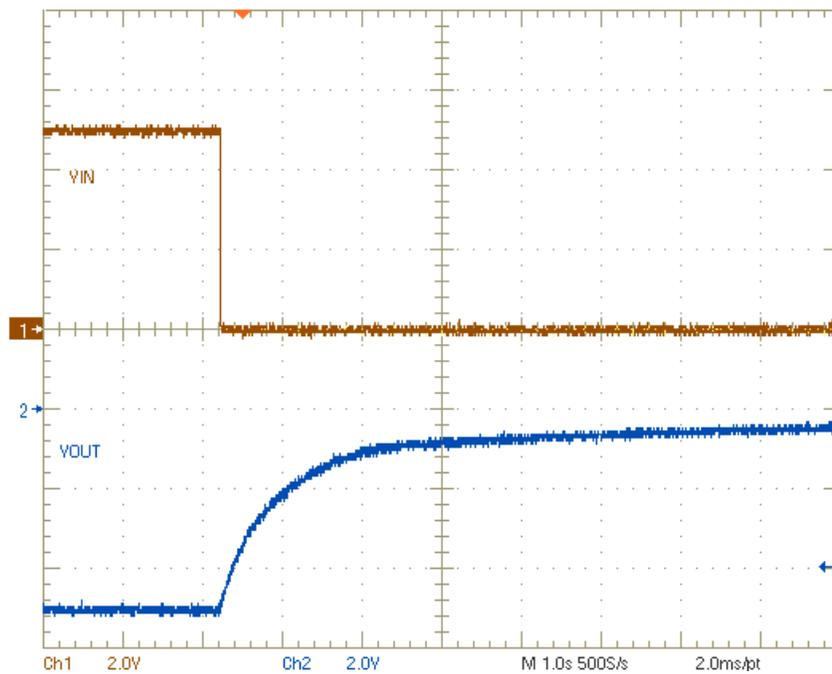
Figure 3-4. Shutdown with No Load
