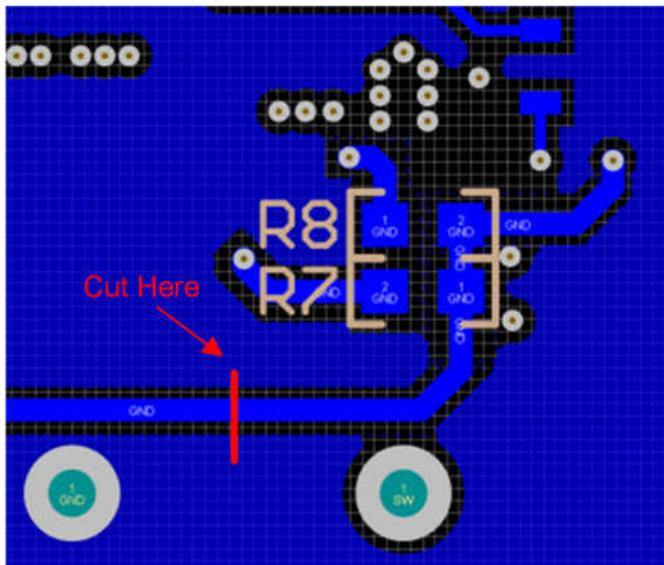
Figure 1-2. Loop Response Measurement Modification (Bottom Layer)
