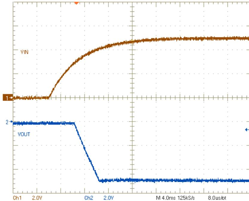
Figure 3-2. Startup with No Load
