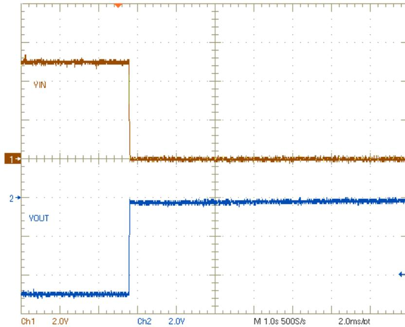
**Figure 3-5. Shutdown with 1A Load**
