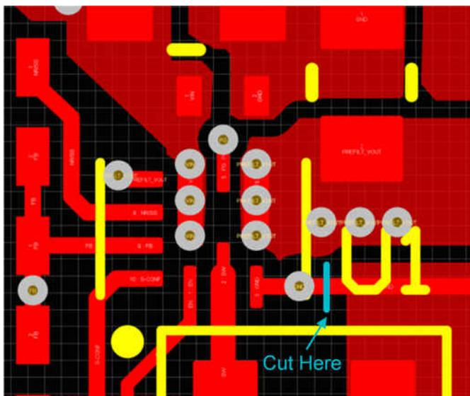
Figure 1-3. Loop Response Measurement Modification (Top Layer)
