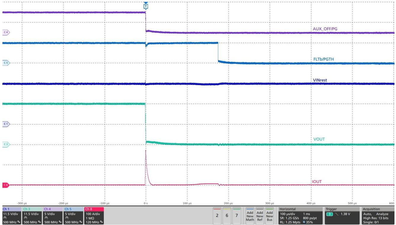
**Figure 5-4. Output Hot-short response of TPS25947xx device at  $V_{in} = 23V$ ,  $C_{out} = 10\mu F$ ,  $ITIMER = OPEN$ ,  $ILIM = 549\Omega$**
