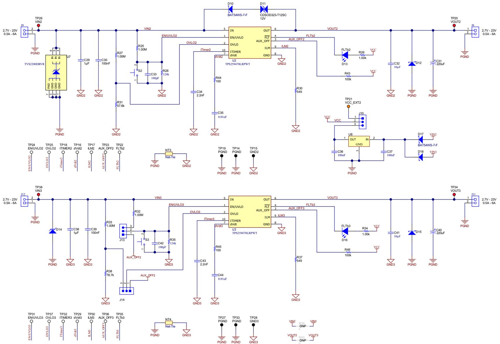
Figure 3-1. TPS25947EVM eFuse Evaluation Board Schematic
