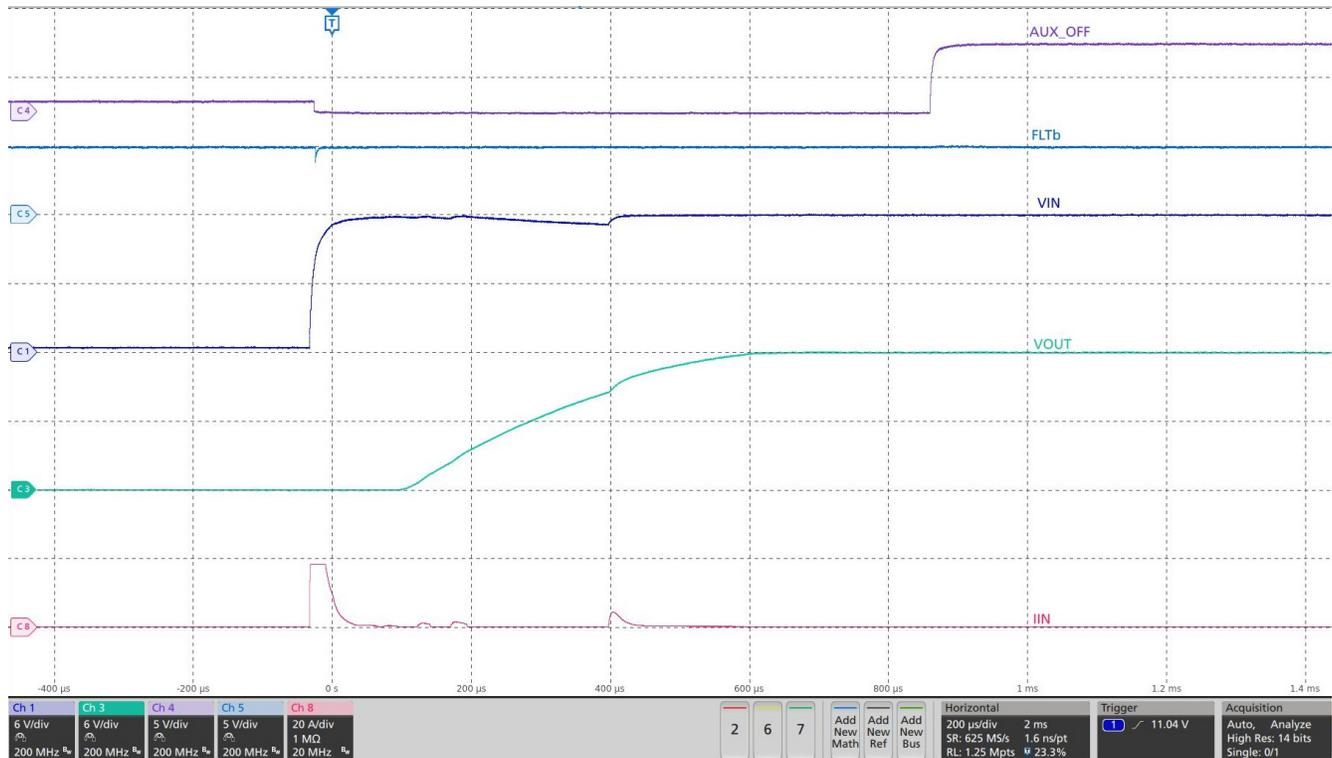
**Figure 5-2. TPS25947x Output Rise Profile ( $V_{IN} = 12\text{ V}$ ,  $C_{out} = 10\mu\text{F}$ ,  $C_{dVdT} = \text{OPEN}$ ,  $I_{LIM} = 549\Omega$ , No-load)**
