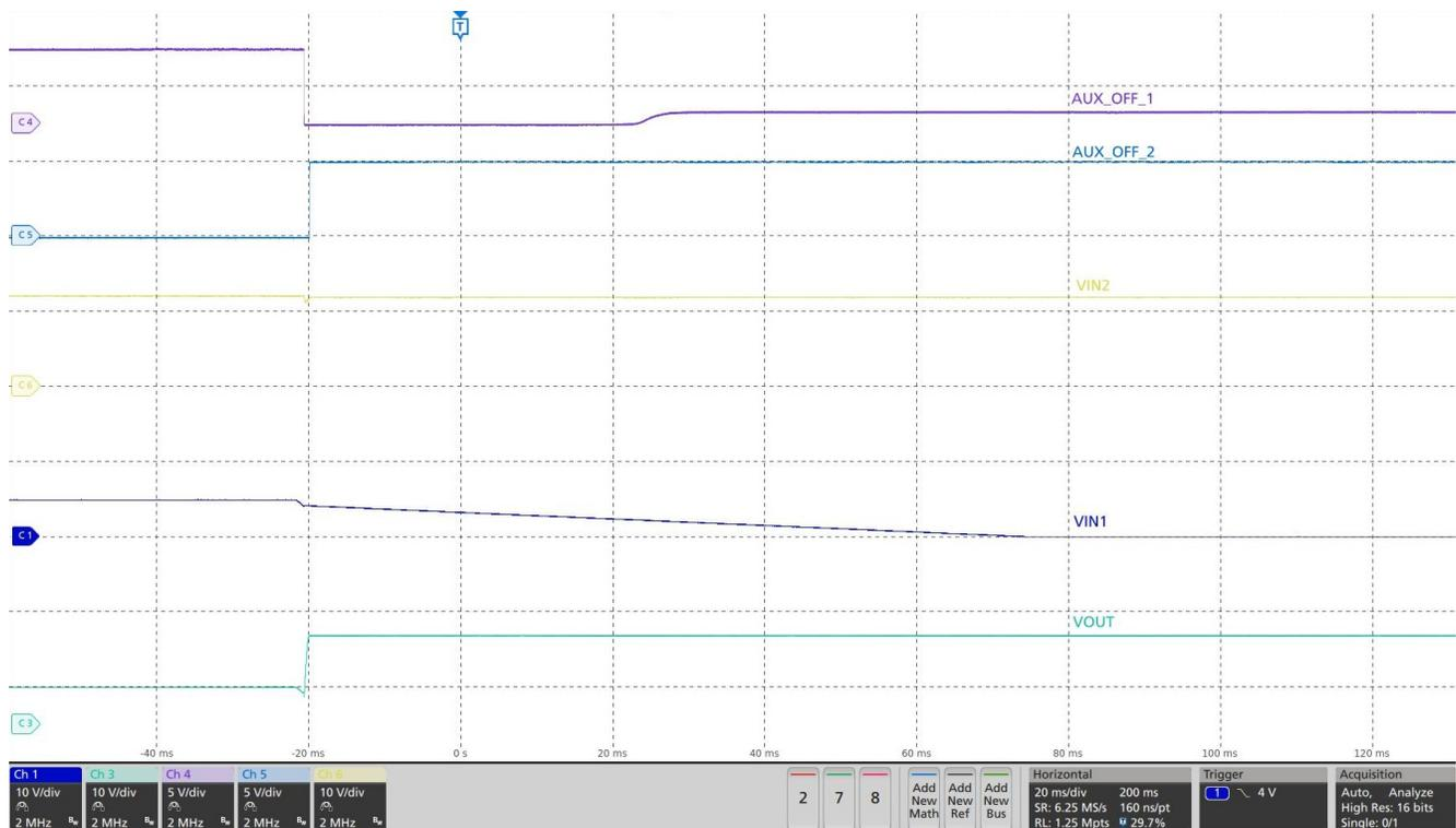
Figure 5-7. Priority PowerMux test on TPS259470x
