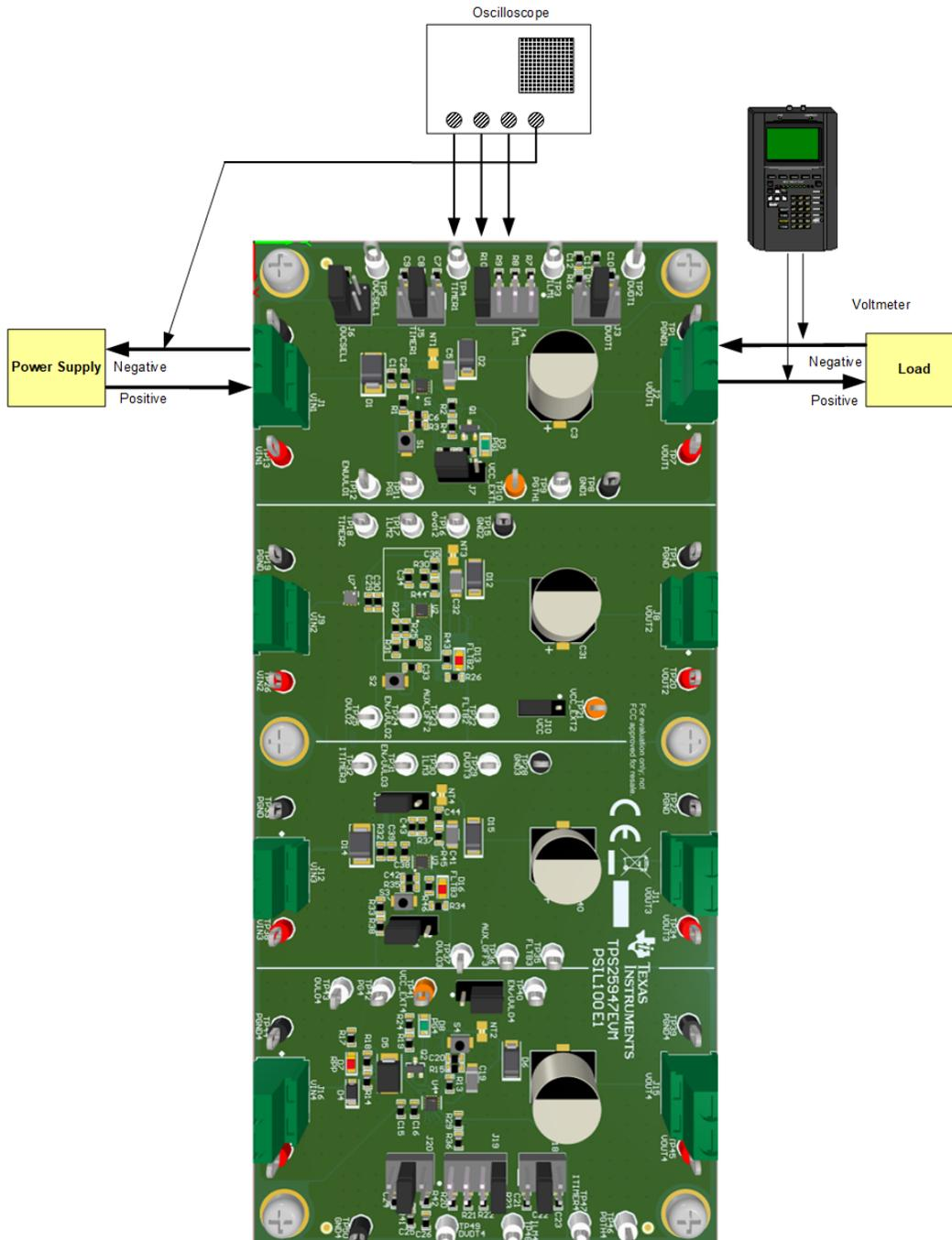
**Figure 5-1. TPS25947EVM Setup with Test Equipment**
