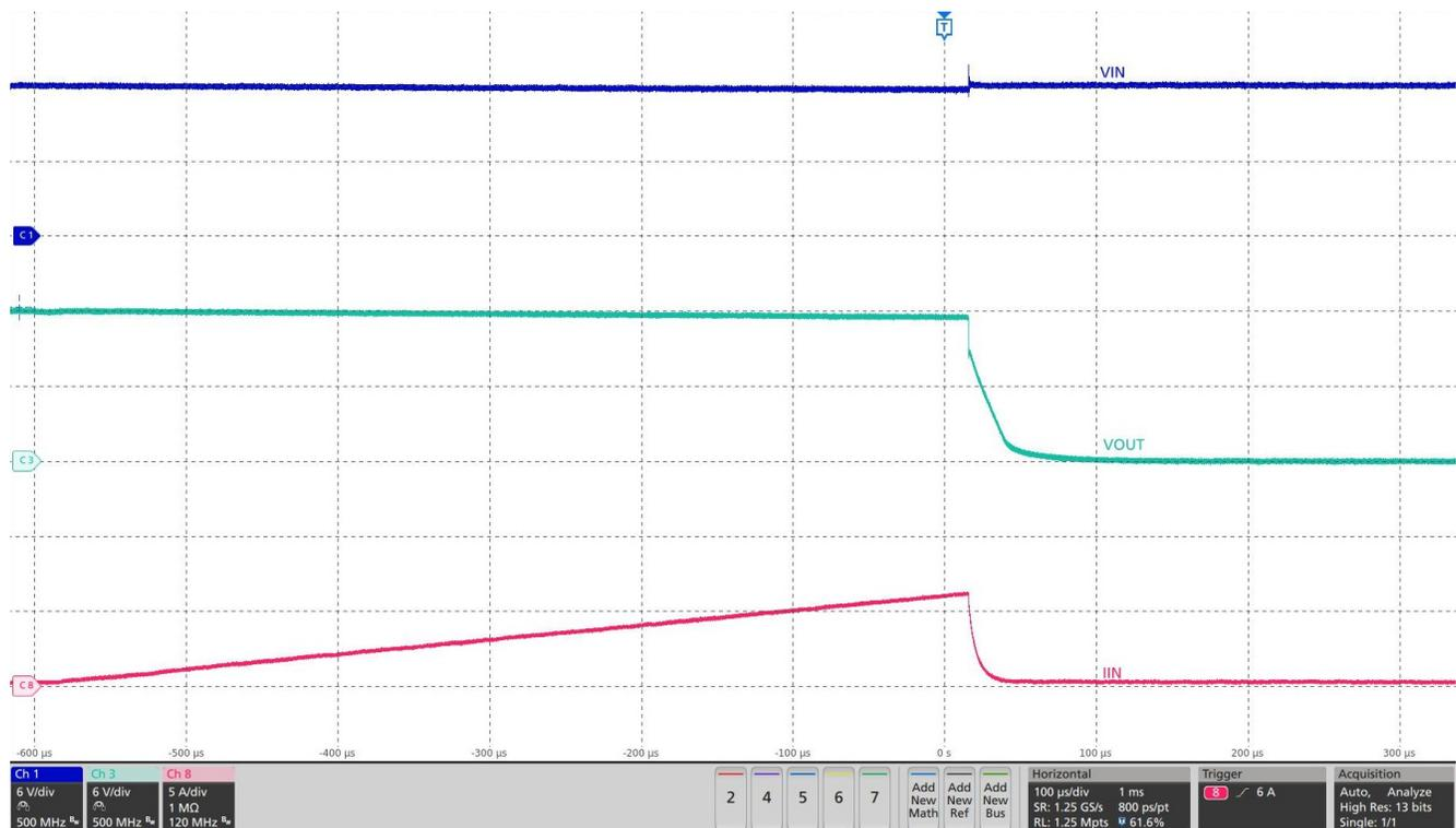
**Figure 5-3. Over Current Response of TPS259474x for 6 A Current Limit Setting**
