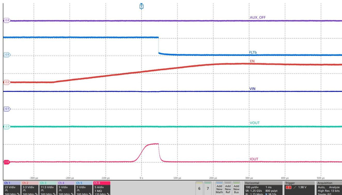
**Figure 5-5. Test Waveform of Wakeup Into Output Short for TPS25947xx Device at  $V_{in} = 23V$ ,  $dV/dt = \text{OPEN}$ ,  $C_{out} = 470 \mu F$ ,  $I_{LIM} = 549 \Omega$**
