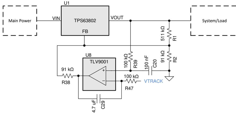
Figure 4-23. Block Diagram for Output Voltage Tracking
