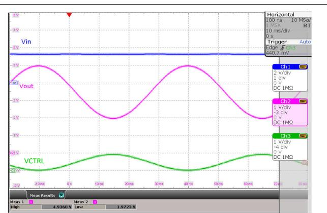
Figure 4-22. Typical Waveform of Analog Dynamic Voltage Scaling
