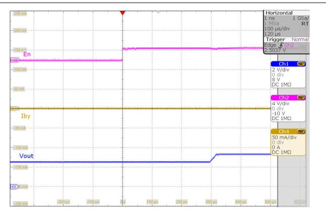
**Figure 4-29. Typical Waveform for Bypass Exit**
