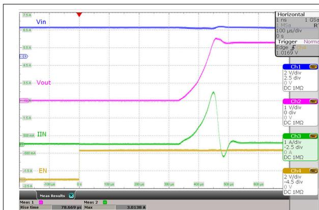
**Figure 4-16. Typical Start-up Standard Operation**
