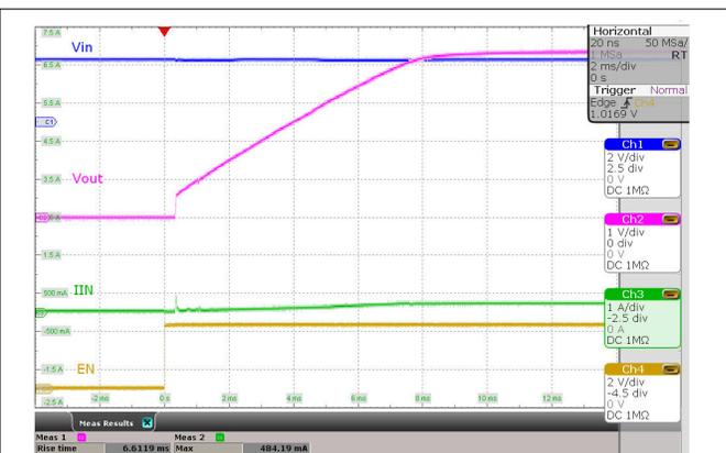
**Figure 4-17. Typical Start-up with Inrush Current Limit and Extended Soft Start**
