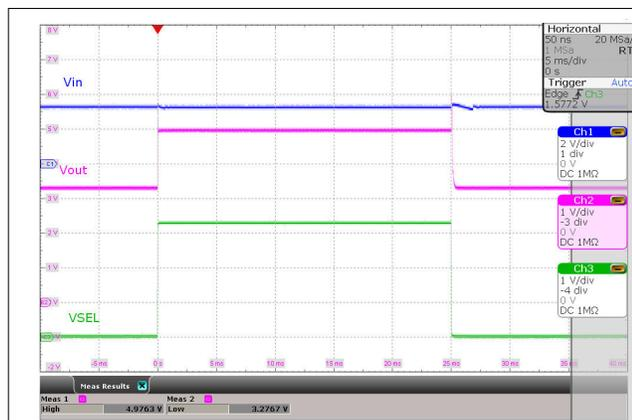
Figure 4-21. Typical Waveform of Two-level Voltage Scaling
