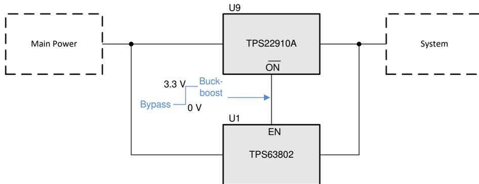
Figure 4-26. Block Diagram for Bypass Mode
