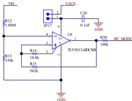
**Figure 4-6. Supercapacitor Voltage Monitor**
