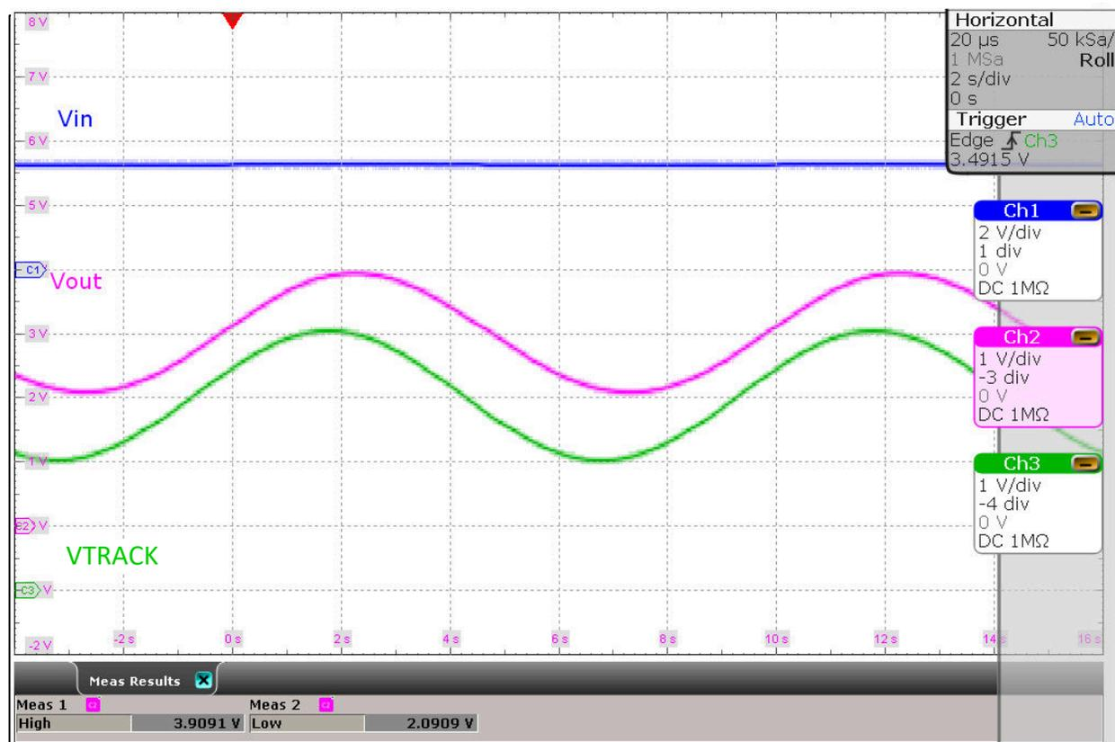
**Figure 4-25. Typical Waveform for Output Voltage Tracking**
