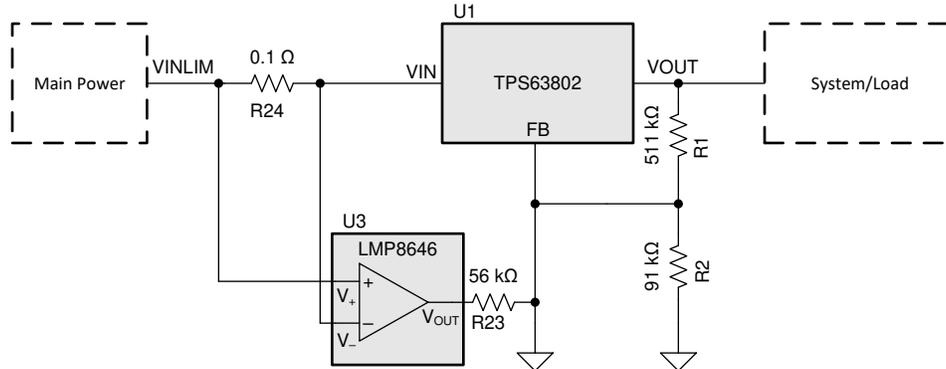
**Figure 4-12. Block Diagram for Input Current Limitation**
