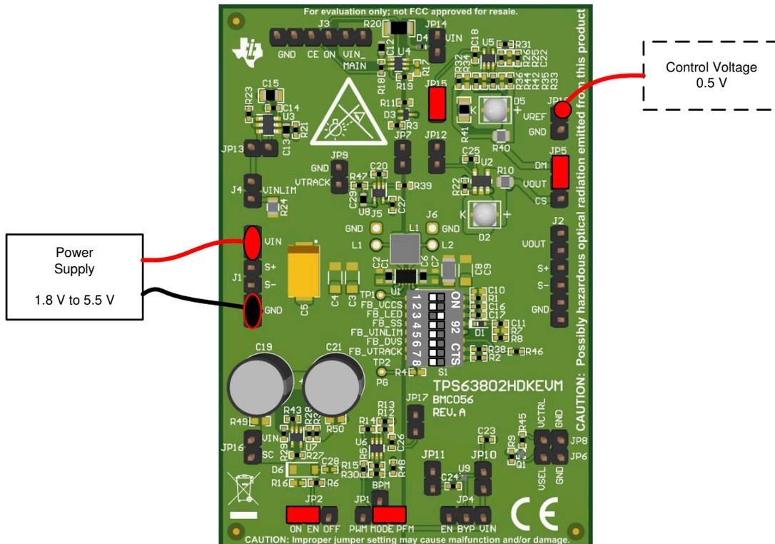
Figure 4-10. Quick Start Connection for High-side LED Driver--Dimming
