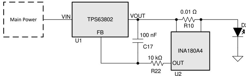
Figure 4-7. Block Diagram for High-side LED Driver -- Constant Current
