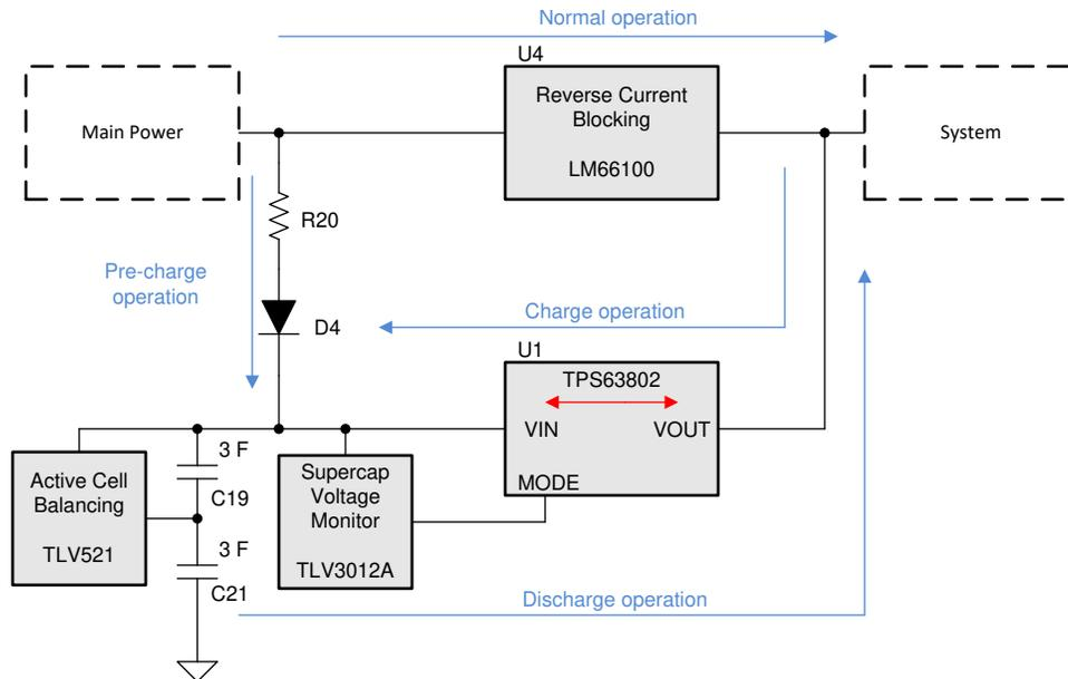
Figure 4-2. Block Diagram for Backup Power
