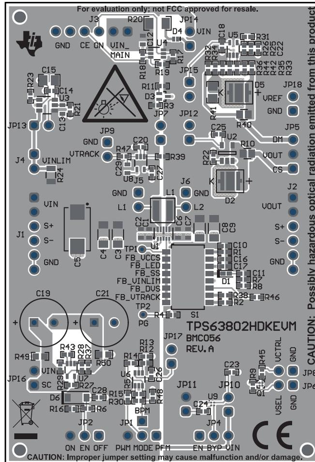
Figure 5-1. Assembly Layer
