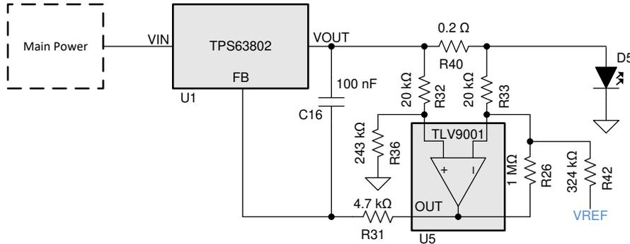
Figure 4-9. Block Diagram for High-side LED Driver with Dimming
