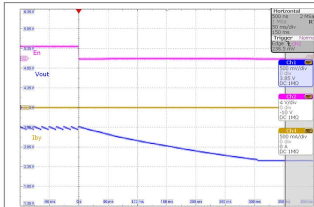
**Figure 4-28. Typical Waveform for Bypass Entry**
