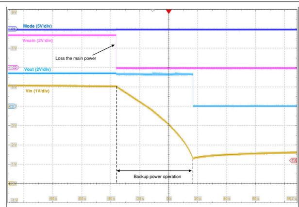
Figure 4-5. Discharge Waveform
