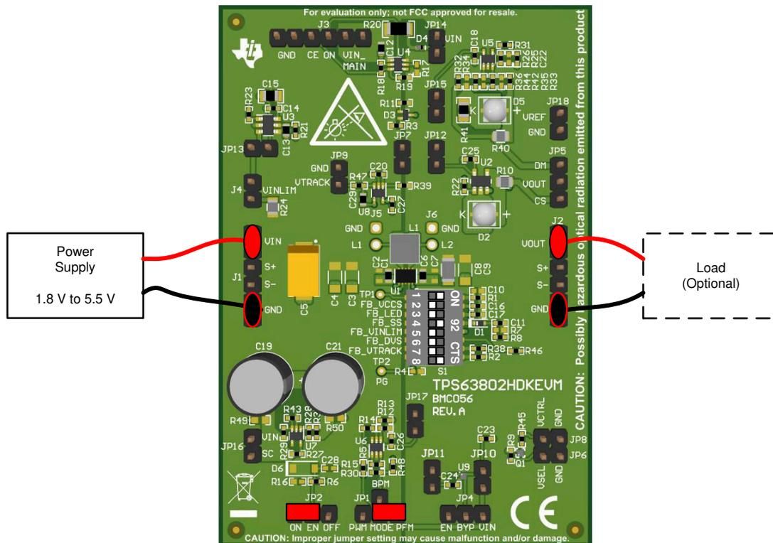
Figure 4-15. Quick Start Connection for Extending Soft Start or Inrush Current Limitation
