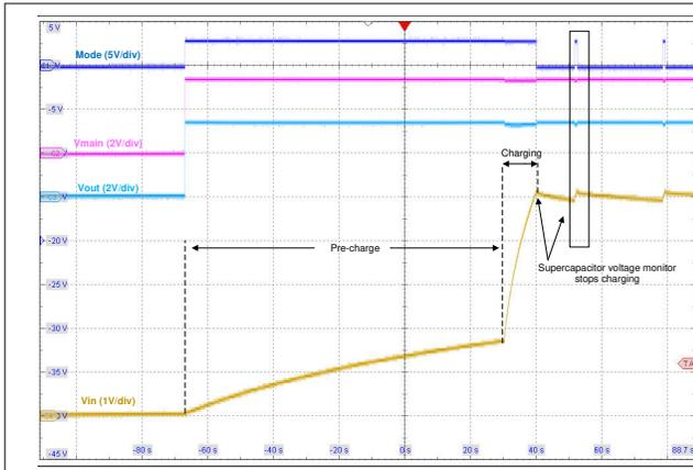
Figure 4-4. Pre-charge Waveform
